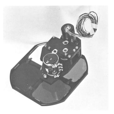
Fig. II-4. Filter-wheel assembly
