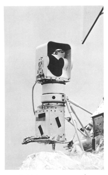
Fig. II-2. Survey camera on spacecraft
