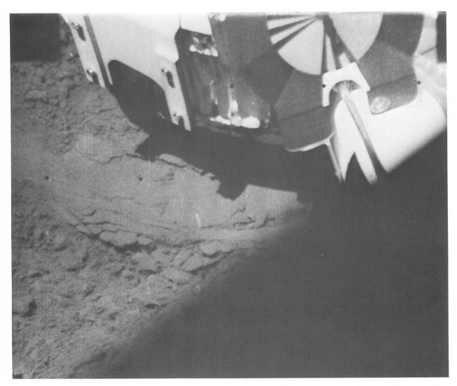
Fig. IV-11. Compressed lunar soil in the bottom of the footpad 2 imprint made during the initial landing (Day 320, 03:35:09 GMT).
