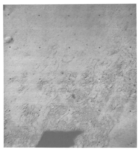
Fig. IV-44. Shallow depressions (area N) in dark, subsurface soil formed by impact of fragments ejected by vernier engine 1 during hop (Day 321, 11:48:31 GMT).
