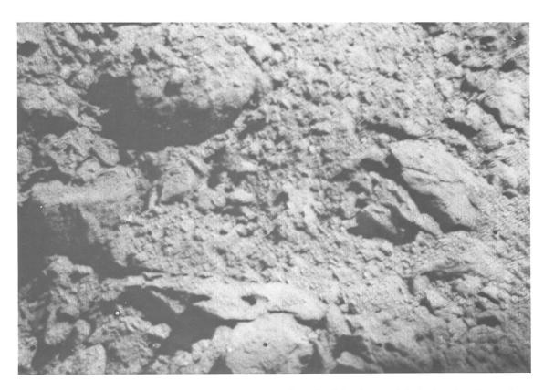
Fig. III-19. Clods of fine-grained surface material disturbed by footpad 2 during landing after the hop made by Surveyor VI early November 17, 1967. Clods are composed of compacted, fine-grained material and bright, rocky chips (Day 323, 06:53:29 GMT).
