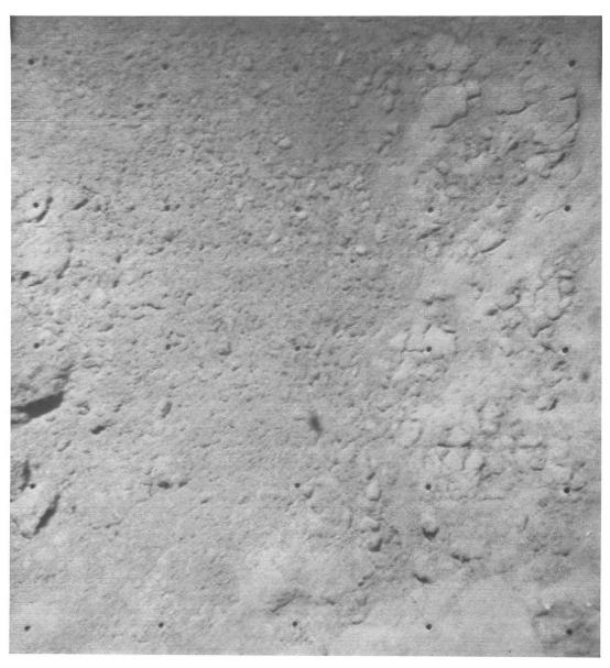
Fig. IV-42. Soil disturbed by vernier engine 1 firing. Soil fragments seen in area L probably have been moved along the surface without being overturned because their tops are formed of light-colored surface soil (Day 321, 11:47:26 GMT).
