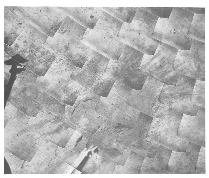
Fig. IV-41. Enlargement of a portion of Fig. IV-31 showing the crushable block 1 impact area and soil disturbance caused by vernier engine 1 during the hop (Days 321 and 322, Catalog 6-SE-23).
