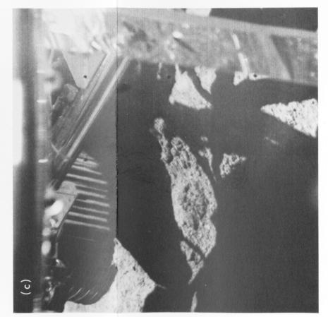
Fig. IV-15. Narrow-angle pictures of crushable block 3 and its impression on the lunar surface. Pictures were taken through the auxiliary mirrors at different sun elevation angles. (a) Sun elevation angle of 15 deg (Day 315, 01:28:20 GMT). (b) Sun elevation angle of 30 deg (Day 316, 07:08:08 GMT). (c) Sun elevation angle of 65 deg (Day 319, 03:57:13 GMT).
