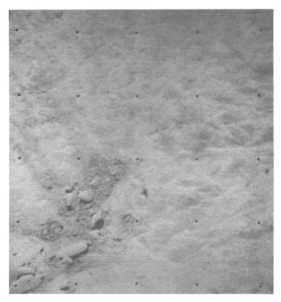
Fig. IV-40. Narrow-angle picture of part of area I (see Fig. IV-31) showing rippled appearance of the surface after vernier engine firing (Day 321, 11:34:18 GMT).
