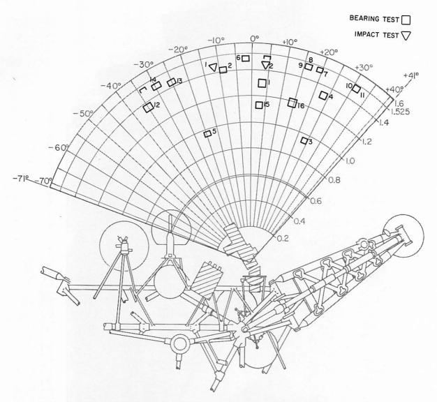
Figure 5-12. — Plan view of surface sampler operations showing location of bearing and impact tests performed.
