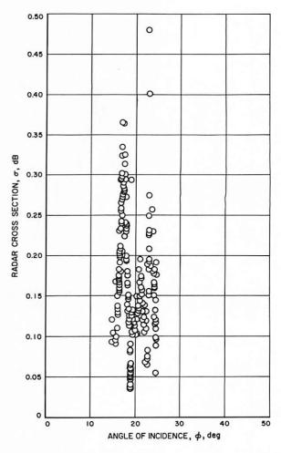
Figure 7-7. — Beam 3 radar cross section, computed from the measured signal strengths as a function of incidence angle.
