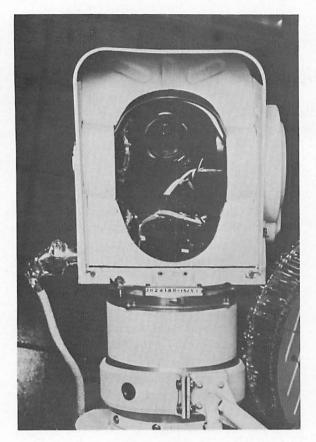
FIGURE 3-1. — Surveyor VII television camera hood and mirror assembly. The mirror is open and reflects the image of the lens and filter-wheel assemblies. The hood, mirror, and filter-wheel assembly rotate in azimuth as a unit.
