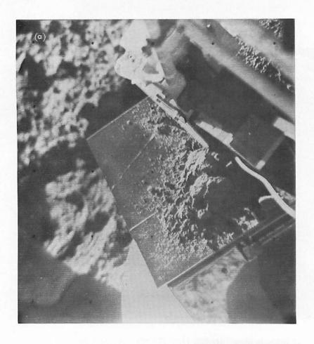
FIGURE 5-31. — (a) Lunar soil dropped on the sensor-head thermal mirror (day 022, 11:03:29 GMT). (b) After redeployment of sensor head, showing soil movement (day 022, 11:31:42 GMT).
