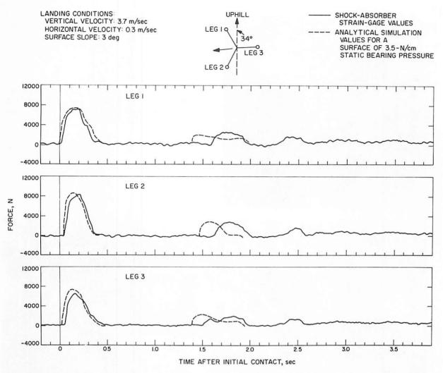
FIGURE 4-21. — Comparison of Surveyor VII landing data with analytically obtained shockabsorber force/time histories.
