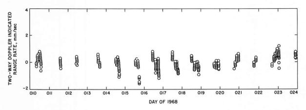
FIGURE 10-3. — Surveyor VII, DSS-42 (Canberra, Australia). First lunar day, O — C residual set (one data point/min). DE 29/LE 5 was used.
