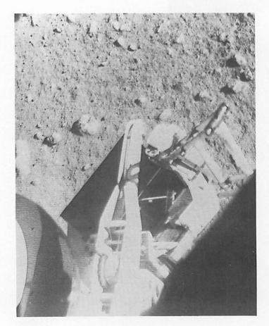
Figure 5-16. — The surface sampler is shown forcing the sensor head against the helium tank, preparatory to applying a downward force to free it (day 012, 06:57:30 GMT).
