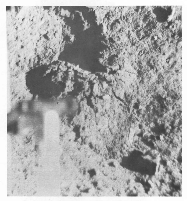
FIGURE 5-26. — Results of bearing test 1 (day 011, 04:09:54 GMT).
