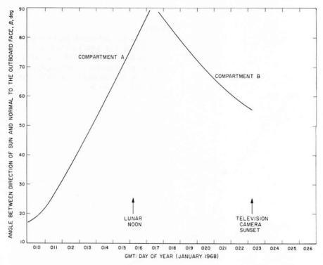
Figure 6-14.—Angle between direction of Sun and normal to outboard plane of compartments.
