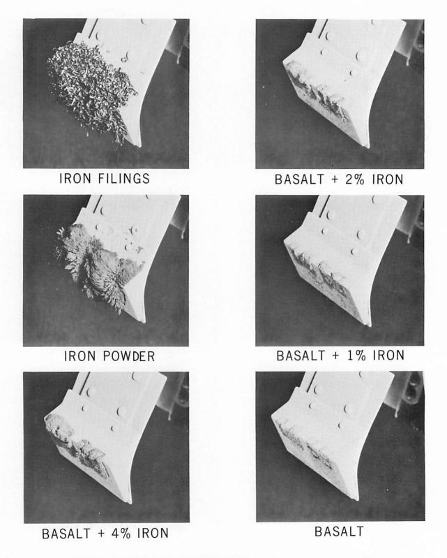
Figure 7-26. — Laboratory studies of surface-sampler magnets impacting in coarse iron filings, powdered iron, and various volumetric percentage additions of powdered iron to basalt powder (37 to  $50_{\mu}$ ).
