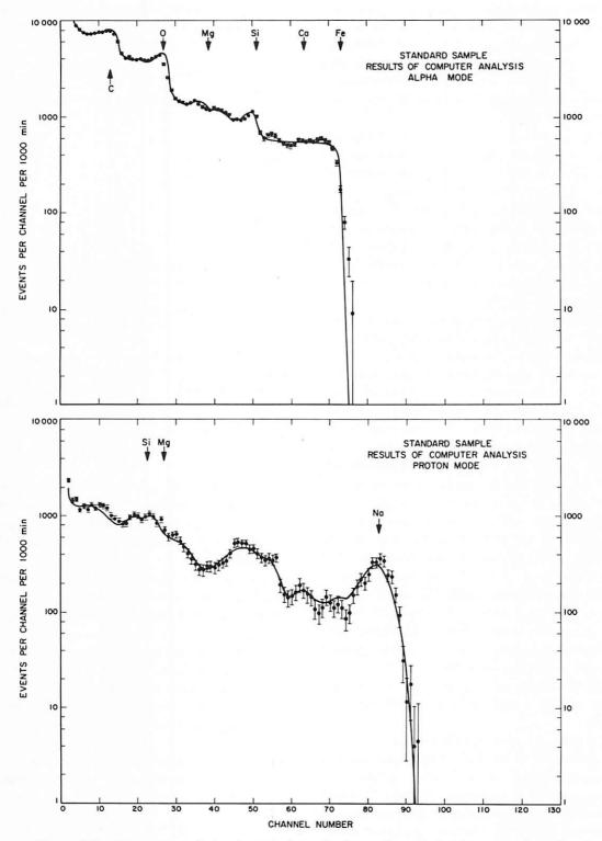
Figure 8-7. — Computer analysis of standard-sample data. The calculated spectra (smooth curves), using an eight-element library, are compared with the data (points with  $(1_{\sigma})$  error bars) taken during 5.0 hours of analysis of the standard sample on the Surveyor VII mission on the Moon. The background (fig. 8-5) has been subtracted before the comparison is made.
