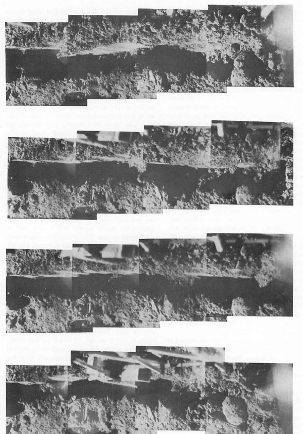
Figure 5-28. — Four mosaics of trench 2, each after a successive pass through the trench, showing trenching progress, left to right (Catalog 7-SE-17).
