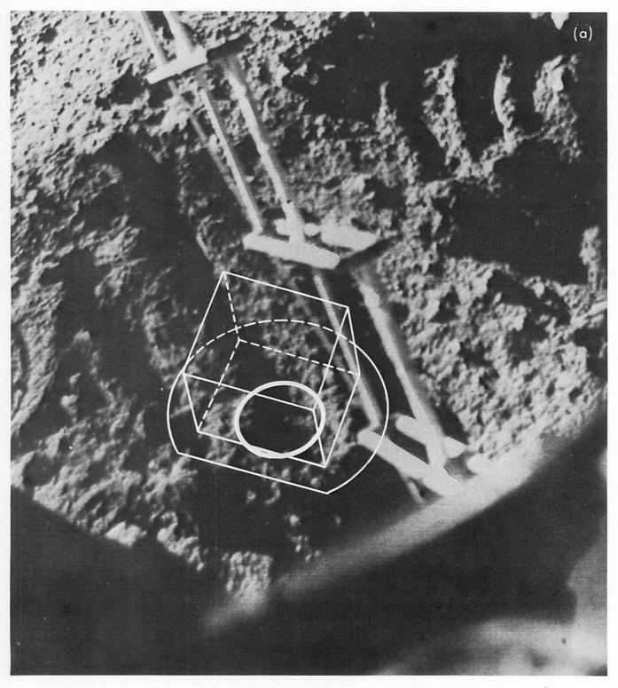
Figure 8-4. — (a) Sample 3, an area of the lunar surface trenched by the surface sampler, later analyzed by means of the Surveyor VII alpha-scattering experiment. (b) The Surveyor VII alpha-scattering instrument on sample 3 (day 022, 11:51:02 GMT).
