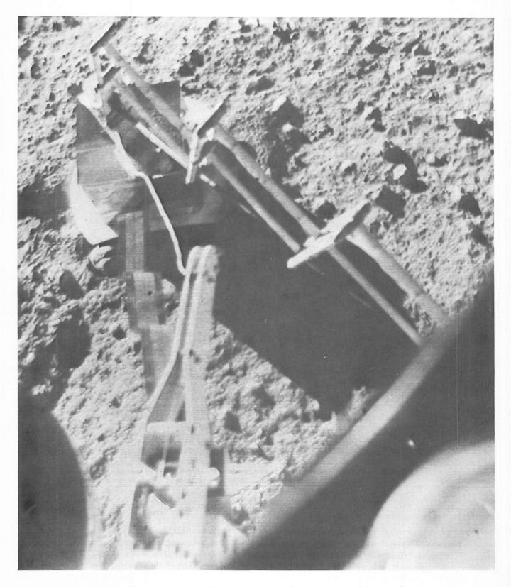
Figure 5-23. — Surface sampler nearing final position in deploying sensor head to second sample on the lunar surface (day 021, 11:44:53 GMT).
