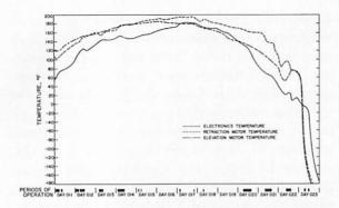
FIGURE 5-10. — First lunar day surface sampler temperatures. Periods of operation are noted by the bars at bottom of figure.
