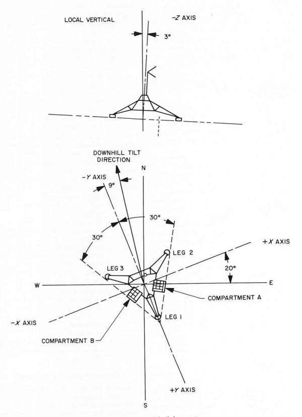
Figure 6-5. - Surveyor VII landed orientation.
