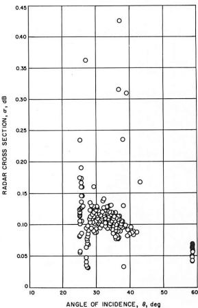
Figure 7-5. — Beam 1 radar cross section, computed from the measured signal strengths as a function of incidence angle.
