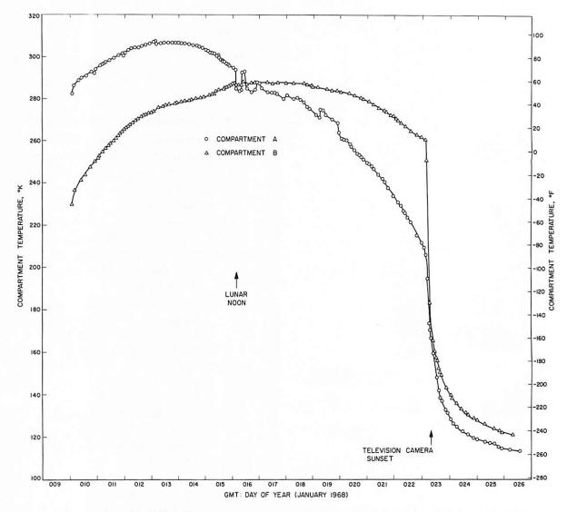
FIGURE 6-10. - Temperatures of outboard face of compartments A and B.
