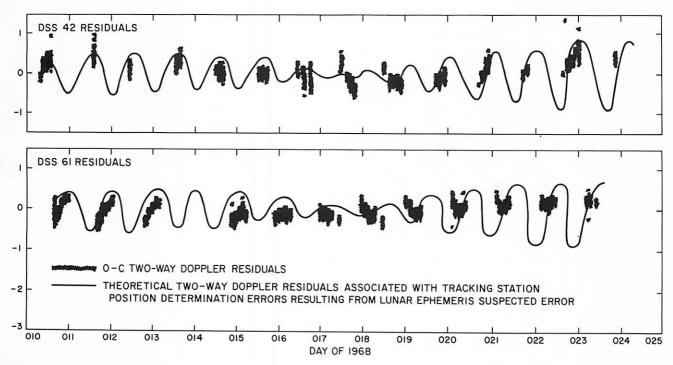
Figure 10-12. — Surveyor VII, DSS-42 and DSS-61. Two-way doppler O — C residual set versus suggested ephemeris-dependent tracking station position error. DE 29/LE 5 was used, coupled with refraction refinement.
