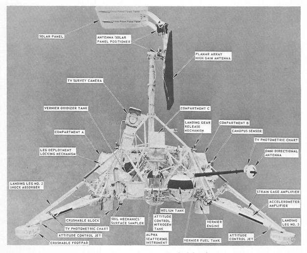
FIGURE 2-1. - Surveyor VII spacecraft - landed configuration.
