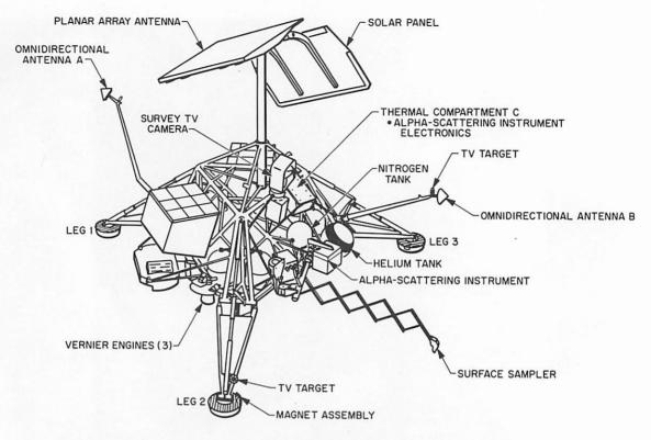
Figure 5-3. — Surveyor VII spacecraft configuration showing surface sampler fully extended. The alpha-scattering instrument is in the stowed position.
