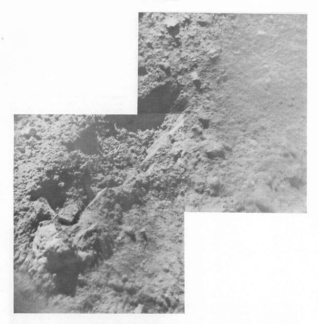
Figure 5-19. — Mosaic of trench 1. Note the irregular shape and shallow depth of the trench (day 019, 20:00:01 and 20:00:59 GMT).
