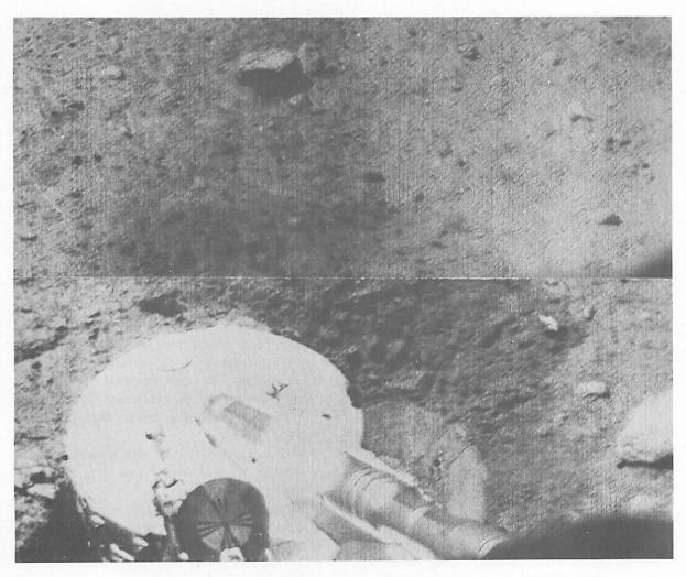
Figure 3-43. - Dark material ejected by the impact of footpad 2 during the Surveyor VII landing (day 015, 08:21:21 and 08:21:27 GMT).
