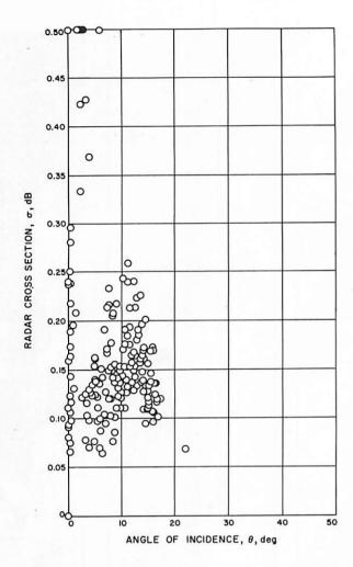
FIGURE 7-8. — Beam 4 radar cross section, computed from the measured signal strengths as a function of incidence angle.
