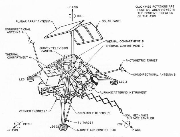
FIGURE 4-1. - Surveyor spacecraft configuration and coordinate system.
