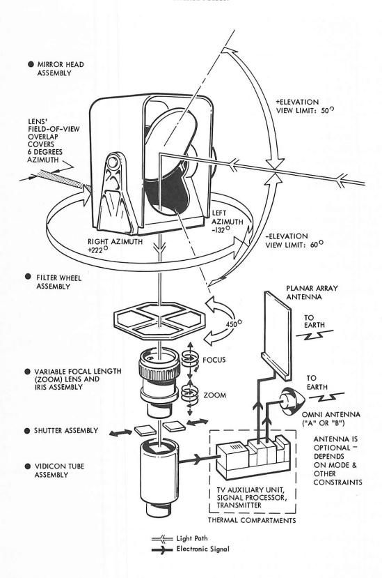
FIGURE 2-3. - Schematic diagram of television and communications subsystems.
