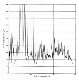
Figure 7-4. — Beam 4 radar cross section, computed from the measured signal strengths as a function of time to touchdown.
