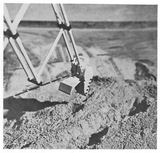
FIGURE 7-15. — Surface sampler with magnets in laboratory studies in basalt powder. Note the magnetic material that outlines the magnet.
