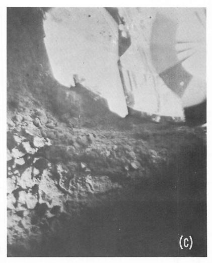
FIGURE 4-10. — Ejected material on the near side of footpad 2, shown under different lighting conditions. A circular depression, probably caused by footpad rebound during the second landing impact, can be seen adjacent to the footpad. Soil clumps, fractured on impact after they were ejected by the footpad at landing, can be seen at the lower left. (a) day 013, 10:21:44 GMT. (b) day 020, 18:13:34 GMT. (c) day 022, 16:08:35 GMT.
