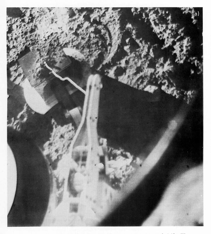
Figure 8-3. — (a) The Surveyor VII alpha-scattering instrument on sample 2 (day 022, 10:38:51 GMT). (b) Sample 2, a lunar rock, after it was analyzed by means of the Surveyor VII alpha-scattering experiment.
