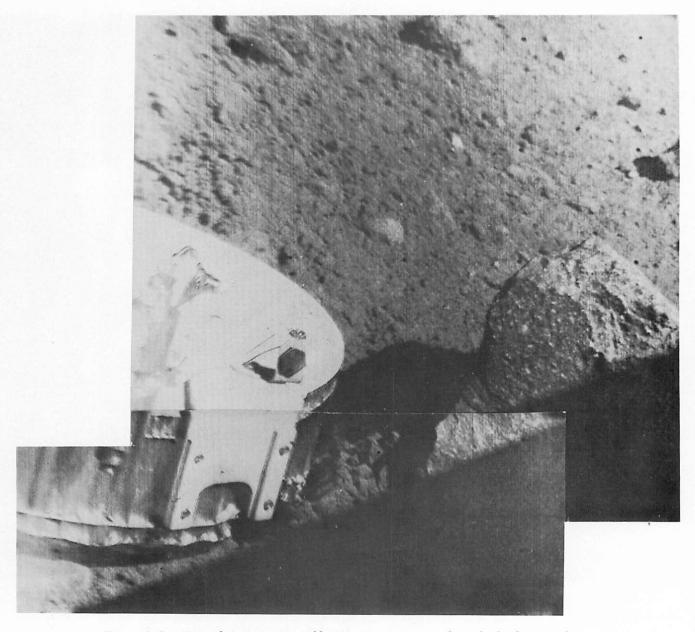
Figure 7-18. — Footpad 3 magnet assembly. No contact was made with the lunar surface material because of insufficient surface penetration.
