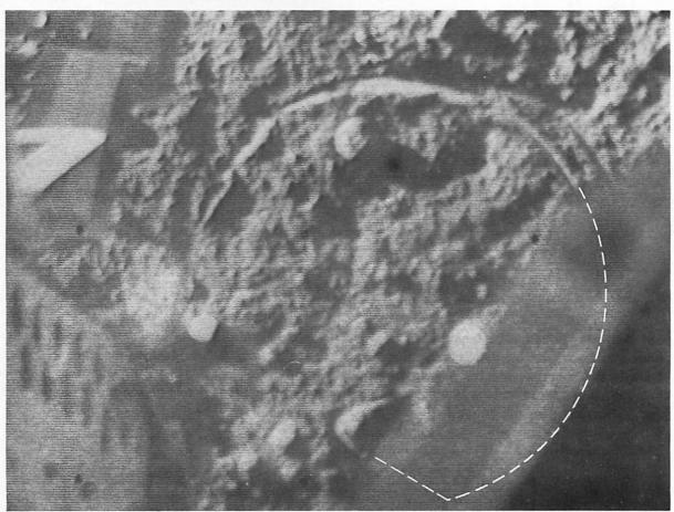
Figure 4-23. — Wide-angle picture showing the discontinuous annular impression made by the sensor head during deployment to the first sample position. The size of this imprint was used in estimating the bearing strength of the topmost layer of soil (day 021; Catalog 7-SE-26).
