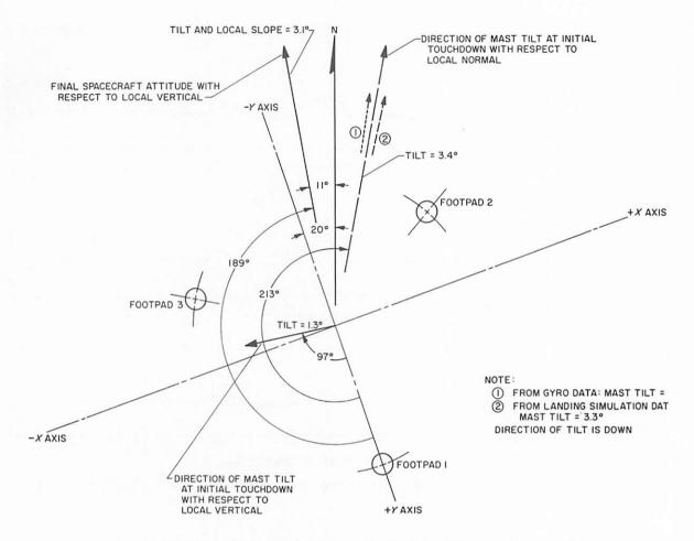
FIGURE 4-3. — Sketch showing landed spacecraft attitude, local slope, and lunar north.
