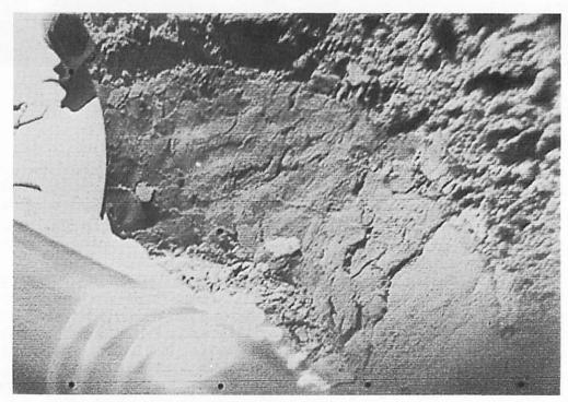
Figure 4-5. — Imprint caused by footpad 2 during first impact, at different lighting angles. The fine-grained nature of the soil is illustrated by the smoothed and flattened wall and floor of the imprint. Cohesiveness of the soil is demonstrated by the presence of open fractures, soil clumps, and side walls that stand at 45° angles.
