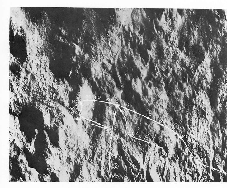
Figure 7-10. — Radar beam traces superimposed on Lunar Orbiter V photograph of Surveyor VII landing site. The touchdown point is indicated by circles; time to touchdown in seconds is indicated by dots.
