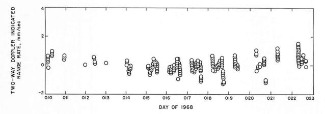
FIGURE 10-2. — Surveyor VII, DSS-11 (Goldstone, Calif.). First lunar day, O — C residual set (one data point/min). DE 29/LE 5 was used.
