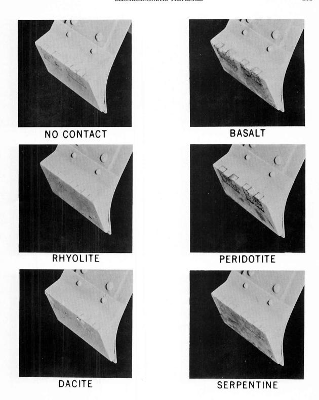
Figure 7-25. — Laboratory studies of surface-sampler magnets impacting in powdered rock types. Note amount of magnetic material collected on pole ends, compared with that observed after the first and second lunar bearing strength tests (figs. 7-20 and 7-21).
