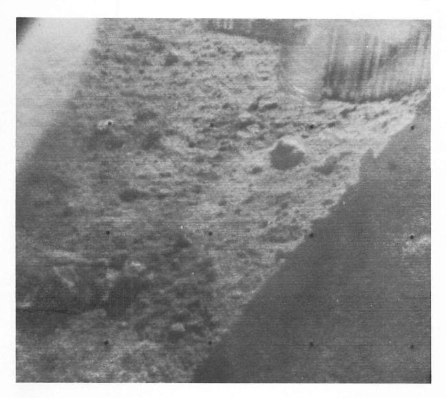
Figure 4-15. — Lunar surface under crushable block 3 and vernier engine 3, visible because of an auxiliary mirror mounted on the spaceframe. Positive evidence of crushable block contact in this area has not been verified; however, spaceframe shadows obscured much of this area throughout the lunar day (day 020, 18:42:14 GMT).
