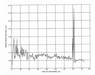
FIGURE 7-2. — Beam 2 radar cross section, computed from the measured signal strengths as a function of time to touchdown.
