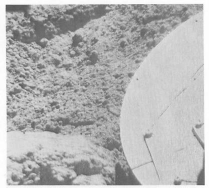
FIGURE 4-11. — A portion of the curved rim that bounds the smooth flat area outboard of footpad 2. The rim may have been formed by soil relaxation during retraction of the shock absorber as the spacecraft came to rest after landing (day 011, 06:10:50 GMT).
