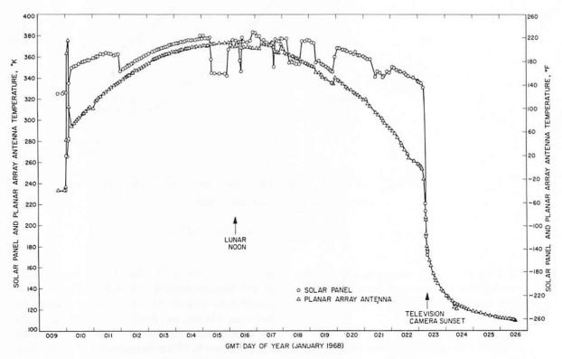
FIGURE 6-15. - Temperatures of solar panel and planar array antenna.
