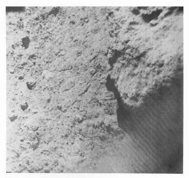
Figure 4-9. – Rock beside footpad 2. The dark soil beside and beyond the rock probably was ejected during landing (day 013, 10:19:18 GMT).
