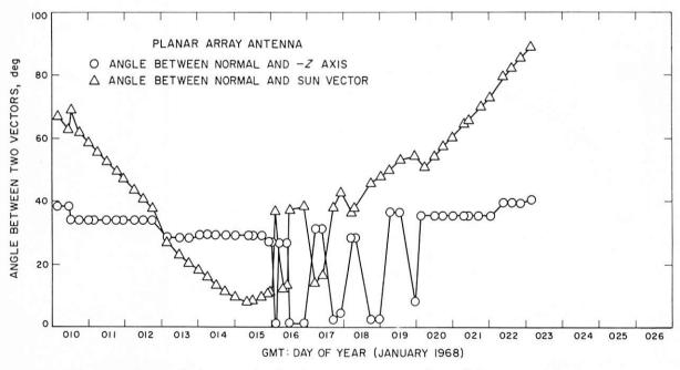
Figure 6-17. — Angle that normal to the planar array antenna makes with Sun vector and  $-\mathbf{Z}$  axis.
