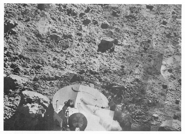
Figure 4-4. — Footpad 2 and surrounding area. Sun elevation was 24°. The footpad imprint just to the right of the footpad, made during first impact, is illuminated by sunlight reflected off the footpad (day 010; Catalog 7-SE-20G).
