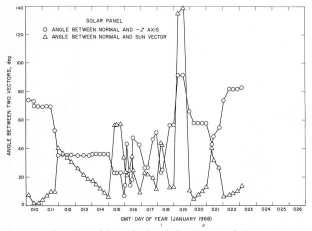
Figure 6-16. — Angle that normal to solar panel makes with Sun vector and -Z axis.
