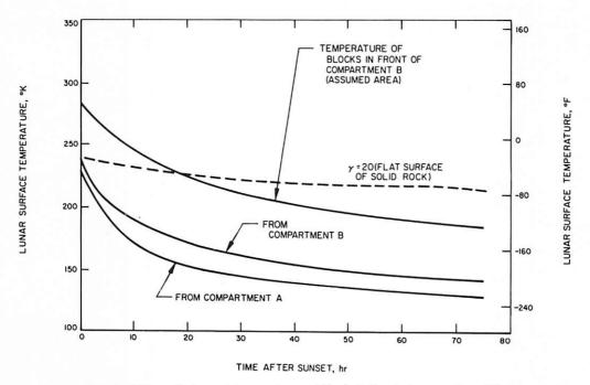
FIGURE 6-21. — Postsunset temperatures of blocks in front of compartment B.
