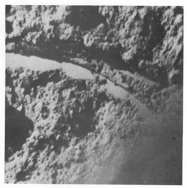
Figure 4-25. — Enlargement showing smooth surface of sensor head imprint at the first sample position; see fig. 4-23 (day 021, 21:53:37 GMT).
