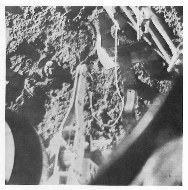
Figure 5-24. — Surface sampler in process of moving sensor head from second to third lunar sample. Note ring around target rock at second sample location (day 022, 11:21:12 GMT).
