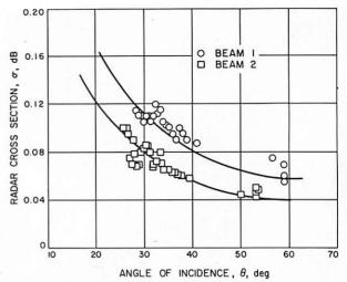
FIGURE 7-9.—Smoothed radar cross section for beams 1 and 2 as a function of incidence angle.
