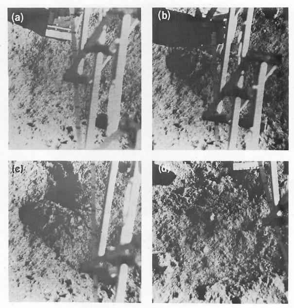
Figure 7-20. — Bearing strength test 1 sequence showing the scoop door. (a) Before contact. (b) During pressure. (c) After contact. The depth of penetration in (b) is about 5 cm. The amount of magnetic material collected on the magnetic pole faces may be compared with laboratory studies (figs. 7-25 and 7-26).
