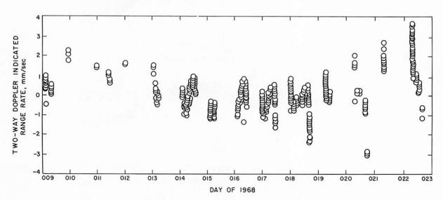
FIGURE 10-9. — Surveyor VII, DSS-11 (Goldstone, Calif.). First lunar day, O — C residual set, (one data point/min). DE 19/LE 4 was used.
