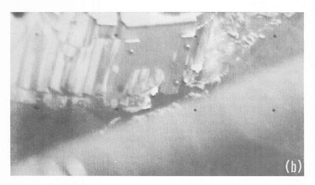
Figure 4-13. — Footpad 3. (a) the hole in the aluminum honeycomb, caused by impact on a rock during landing. A small rock under the footpad can be seen at the left (day 015, 05:40:03 GMT). (b) edges of the broken honeycomb highlighted by the Sun (day 020, 20:25:20 GMT).
