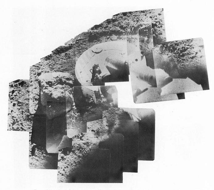
Figure 7-16. — Footpad 2 magnet assembly after landing. The footpad penetration of the surface material was insufficient to produce contact with lunar surface material. Dark mark on magnet side is south pole designation. Fine particles near the bottom are from material acquired during the landing (Catalog 7-SE-7).
