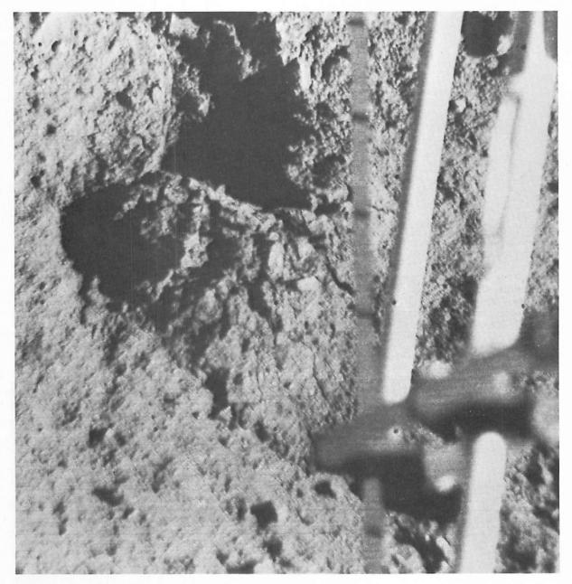
FIGURE 5-13. — Bearing test 1. This picture shows the first surface sampler contact with the lunar surface at the Surveyor VII landing site (day 011, 03:55:42 GMT).
