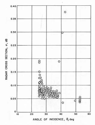
FIGURE 7-6. — Beam 2 radar cross section, computed from the measured signal strengths as a function of incidence angle.
