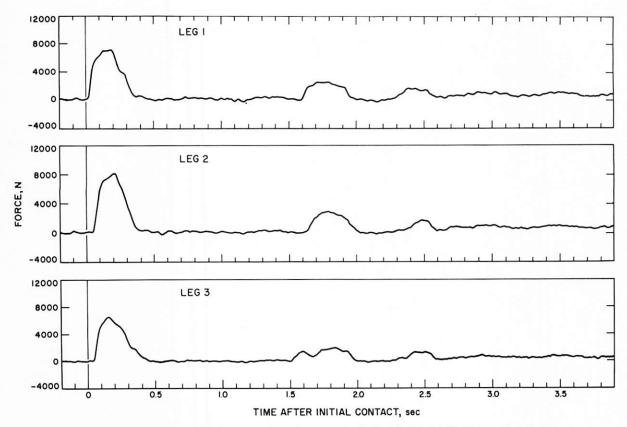
Figure 4-2. — Strain-gage telemetry data showing shock-absorber axial load histories during landing.
