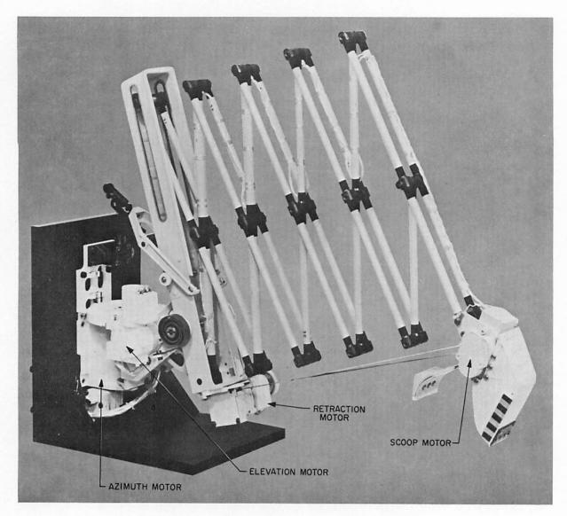
FIGURE 5-1. — Surface sampler on test stand, partially extended.
