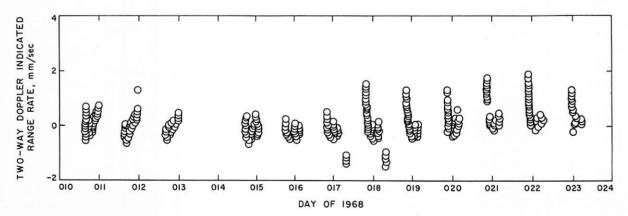
Figure 10-4. — Surveyor VII, DSS-61 (Robledo, Spain). First lunar day, O — C residual set (one data point/min). DE 29/LE 5 was used.
