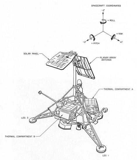
Figure 6-4. - Surveyor spacecraft configuration.
