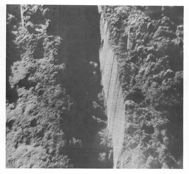
Figure 4-26. — Smooth, vertical wall and the floor of the trench excavated by the surface sampler demonstrates the fine-grained, cohesive nature of lunar soil (day 020, 09:51:50 GMT).
