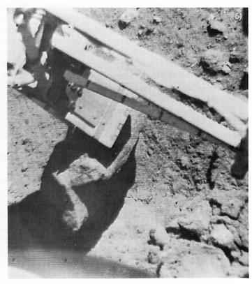
tests 8 and 9 were performed at the same site, just left of bearing point 7, as can be seen in figure 5-12. Bearing test 8 was performed with the scoop closed, using command tape 907, for a total of four 0.5-second lower commands. Figures 5-21(a) and 5-21(b) show bearing test 8 in progress and after removal of the scoop, respectively.
