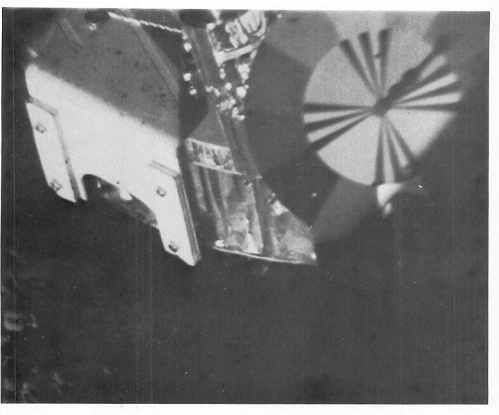
FIGURE 7-17. — Closeup of magnet assembly on footpad 2 after landing. Note the particles on top of the bracket; a few particles also adhere to the lower ends of the poles; these particles may also be caused by the landing disturbance (day 022, 16:10:01 GMT).
