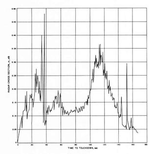
FIGURE 7-3. — Beam 3 radar cross section, computed from the measured signal strengths as a function of time to touchdown.
