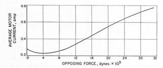
Figure 5-8. — Calibration curve produced from preflight calibration performed at Cape Kennedy, Fla. This curve shows force versus current for the bearing test mode with the surface sampler at 147-cm extension.
