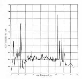
FIGURE 7-1. — Beam 1 radar cross section, computed from the measured signal strengths as a function of time to touchdown.
