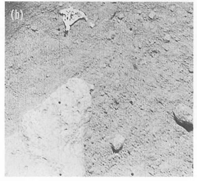
Figure 4-20. — Fibrous-like objects to the right of footpad 2. The bright appearance and unusual shape, unlike that of other fragments on the lunar surface, indicate that the objects probably originated from the spacecraft. (a) day 020, 19:33:56 GMT, computer processed. (b) day 019, 19:42:37 GMT, computer processed.
