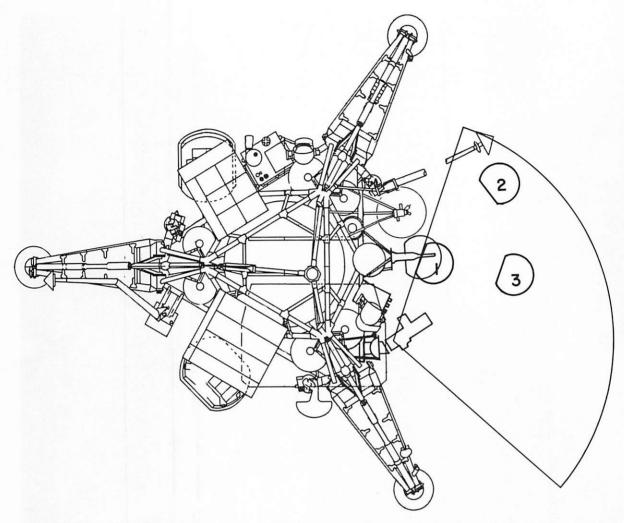
Figure 8-1.—Plan view of Surveyor VII showing the three sample locations of the alphascattering instrument on the lunar surface. The large sector of a circle shows the area of operation of the surface sampler.
