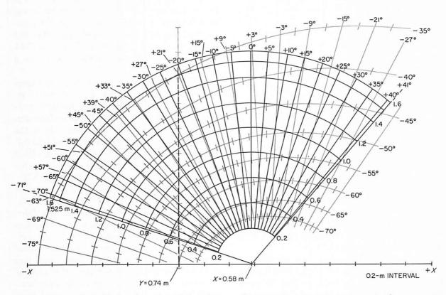
Figure 5-9. — Operational aid used for selecting television camera position to view specific areas of surface-sampler operations.
