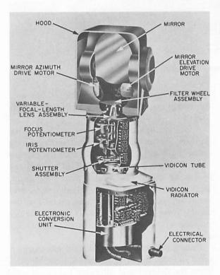
Figure 2-2. - Cutaway view of survey television camera.
