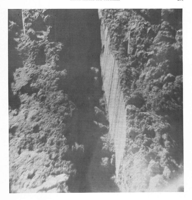
Figure 9-28. — Illuminated sidewall of a trench made in the surface layer by repeated manipulations of the surface sampler (day 020, 09:51:50 GMT).
