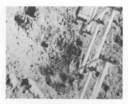
Figure 4-29. — Wide-angle picture of surface sampler just before rock A was dropped; rock A is inside the scoop (day 012, 03:44:17 GMT).
