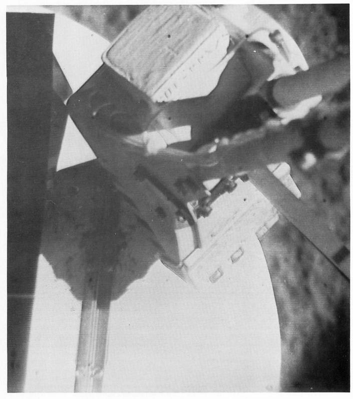
Figure 7-22. — SMSS magnets after two bearing strength tests; compare with figs. 7-25 and 7-26 (day 011, 07:48:26 GMT).
