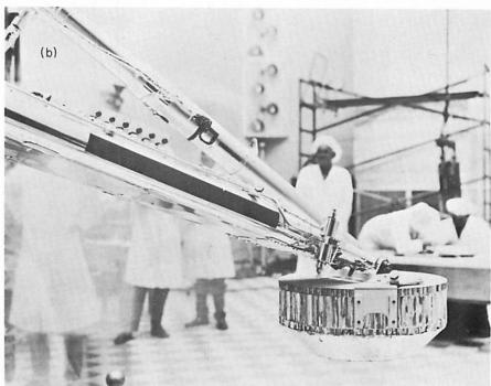
Figure 7-13. — Magnet assembly before flight. The magnetic bar is on the left; the nonmagnetic control bar is on the right. Magnetic flux along the pole edges is about 600 gauss. The control bar has flux readings of less than 0.1 gauss over the surface of the bar. Dark "S" on magnet side indicates the south pole. (a) Footpad 2 assembly. (b) Footpad 3 assembly.
