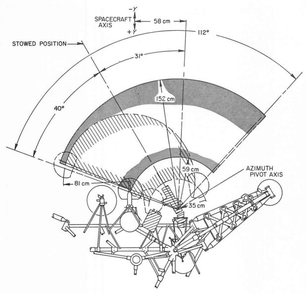
Figure 5-4. — Plan view of surface-sampler area of operations for a nominal surface. The cross hatching indicates the area within which the alpha-scattering instrument sensor head can be manipulated by the surface sampler.
