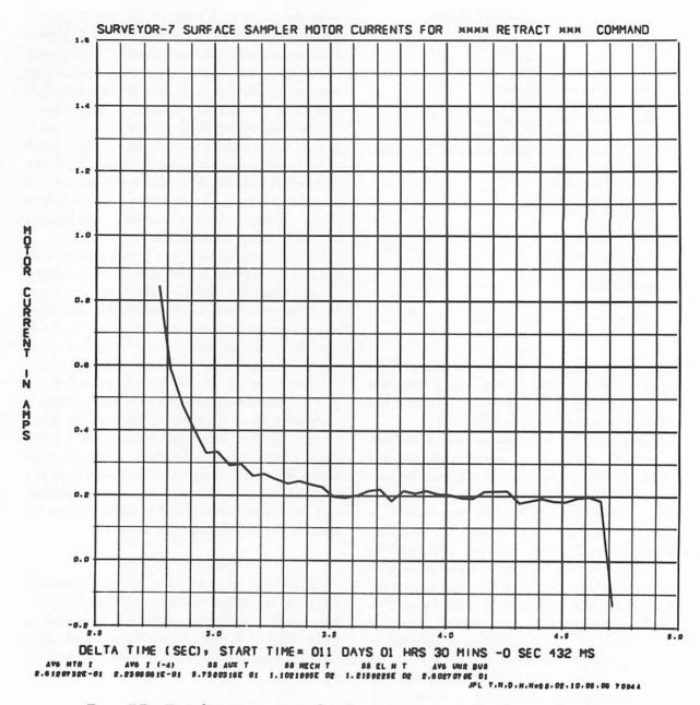
Figure 5-7. — Typical computer output plot of postmission, processed surface-sampler motor current.
