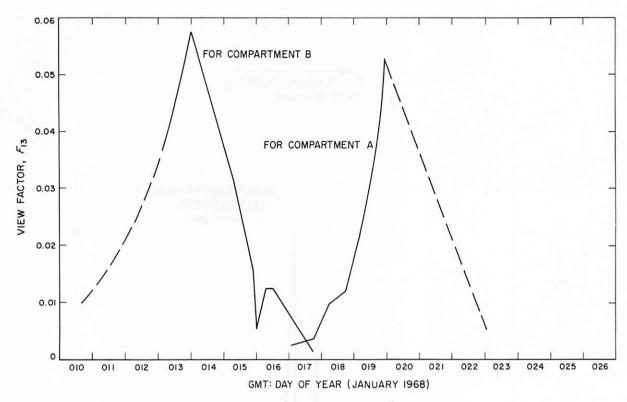
FIGURE 6-12. — View factor, F<sub>13</sub>, from compartment outboard face to the shaded part of lunar surface.
