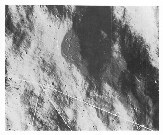
FIGURE 7-11. — Enlargement of part of fig. 7-10. The touchdown point is indicated by the intersection; time to touchdown in seconds is indicated by dots.
