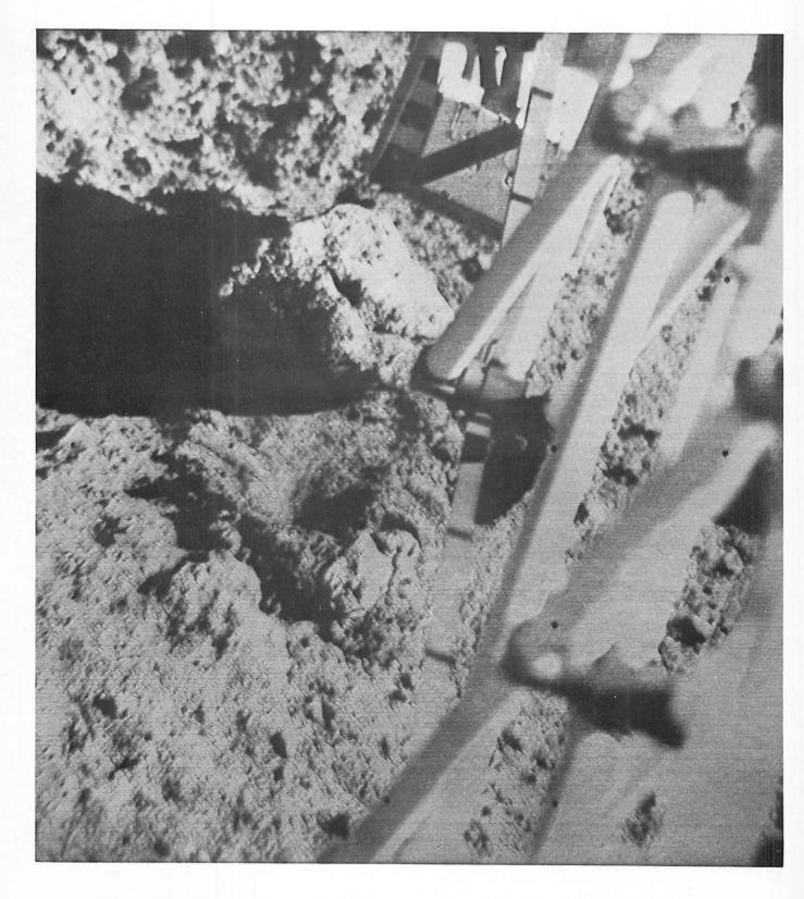
Figure 4-28. — Surface-sampler scoop after initial attempt to pick up rock A. The rock is approximately the same size as the 5-cm width of the scoop (day 012, 02:29:00 GMT).
