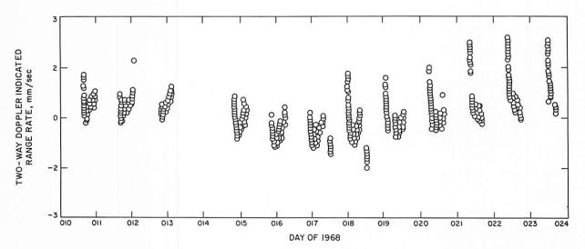
FIGURE 10-11. — Surveyor VII, DSS-61 (Robledo, Spain). First lunar day, O — C residual set (one data point/min). DE 19/LE 4 was used.
