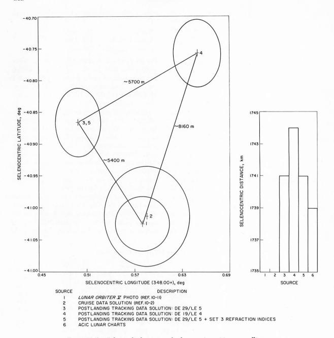
Figure 10-5. - Relative displacements of selenocentric position error ellipses.
