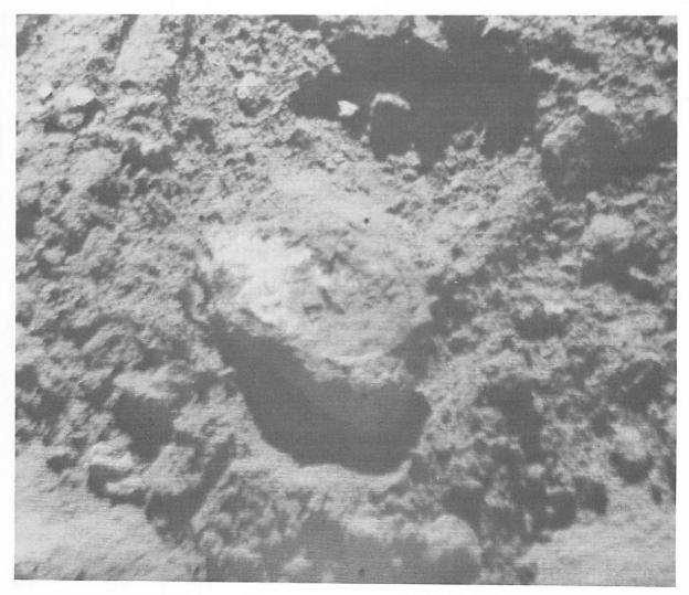
Figure 3-44. — Small fragment, about 6 cm across, turned over by surface sampler on Surveyor VII, exposing dark underside. Part of dark coating has been scraped away by surface sampler (day 018, 06:03:17 GMT).
