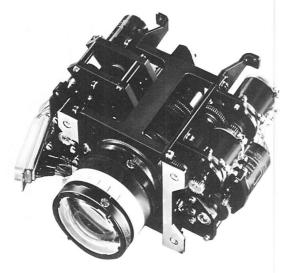
Fig. II-9. Variable-focal-length lens assembly
