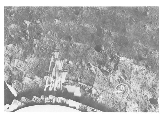
Fig. VII-19. Mosaic of the area in which the surface sampler operated. Bearing strength tests 1 and 2 were in the vicinity of a; a rock thought worthy of testing was spotted at location b.
