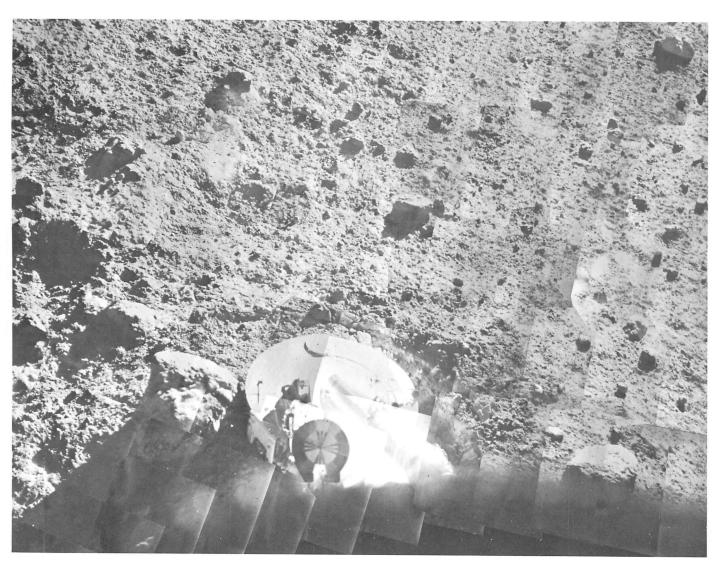
Fig. IV-4. Footpad 2 and surrounding area. Sun elevation was 24 deg. The footpad imprint just to the right of the footpad, made during first impact, is illuminated by sunlight reflected off the footpad (Day 010; Catalog 7-SE-20G).
