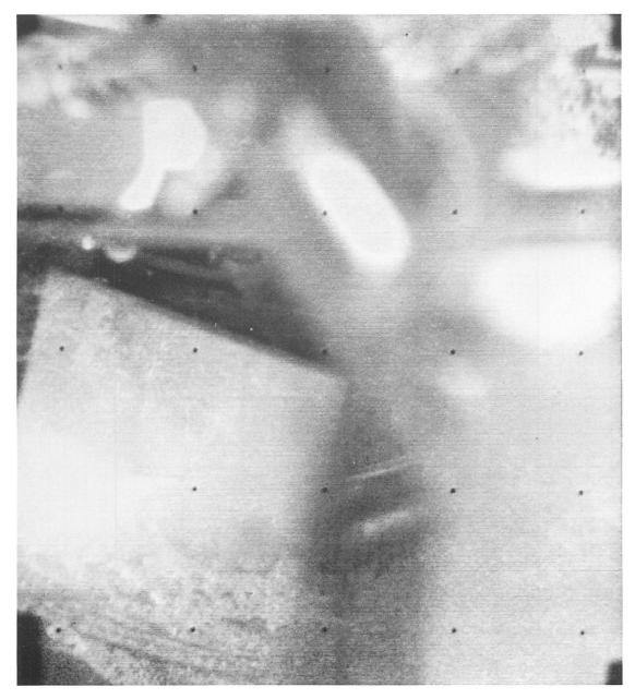
Fig. IV-18. Upper half of the crushable block 2 auxiliary mirror. The bright glare is caused by sunlight striking a thin layer of fine soil that was deposited on the mirror during the landing. The lunar surface area is the same as in Fig. IV-14c; the crushable block 2 imprint can be seen in both pictures (Day 020, 18:42:48 GMT).
