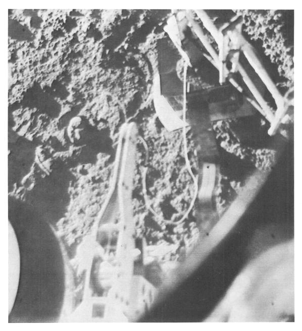
Fig. V-24. Surface sampler in process of moving sensor head from second to third lunar sample. Note ring around target rock at second sample location (Day 022, 11:21:12 GMT).
