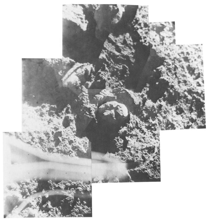
Fig. IV-24. Mosaic showing the second sample position. Note short, wide imprint at upper left and long, narrow imprint at lower right (Day 022, Catalog 7-SE-25).
