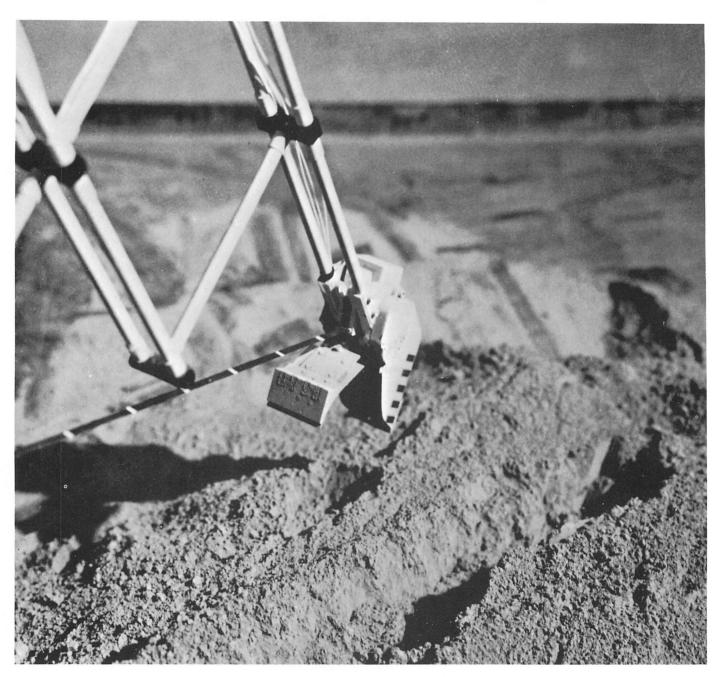
Fig. VII-15. Surface sampler with magnets in laboratory studies in basalt powder. Note the magnetic material that outlines the magnet.
