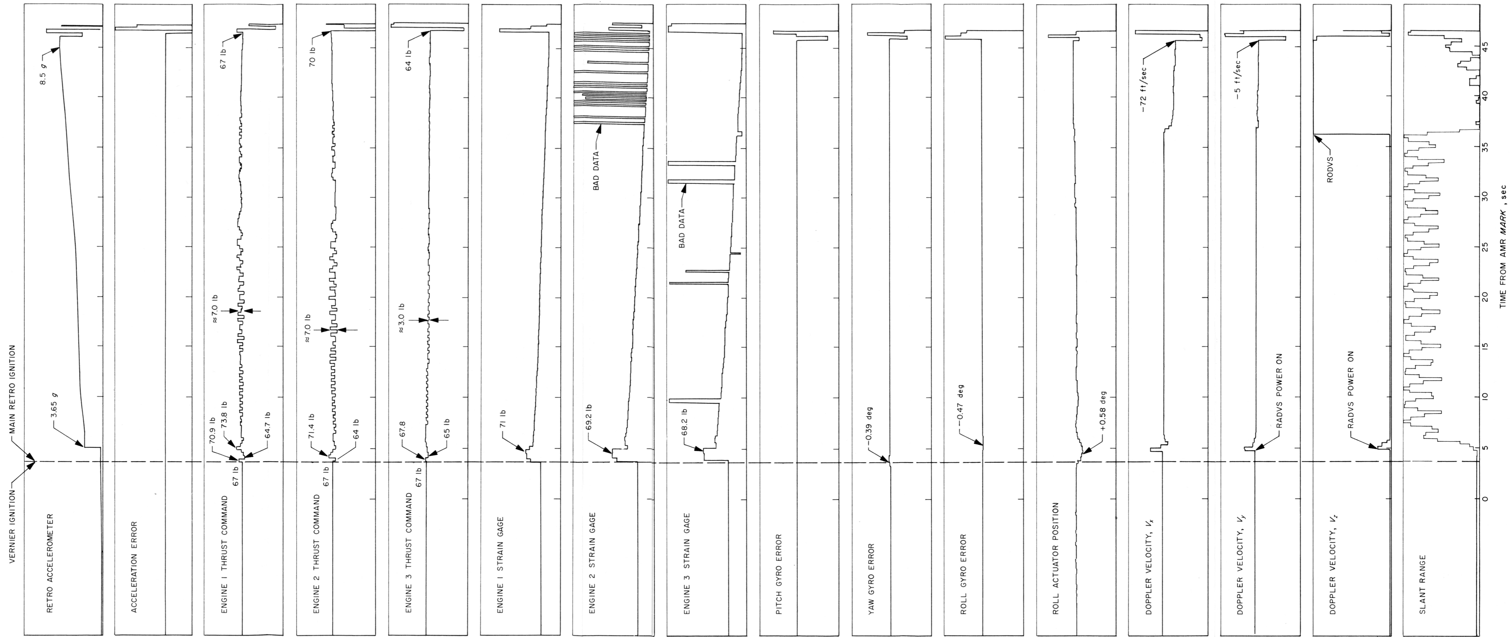
Fig. IV-25. Critical flight control signal recordings during main retro phase
