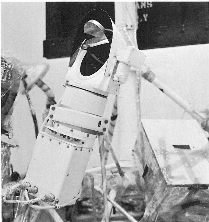
Fig. II-2. Survey camera on Surveyor spacecraft
