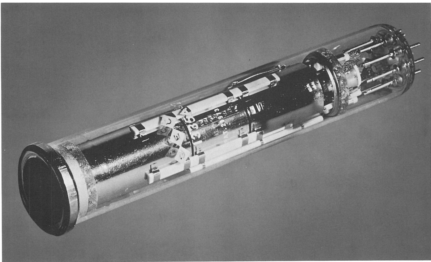
**Fig. II-8. The 2.58-cm vidicon for survey camera**
