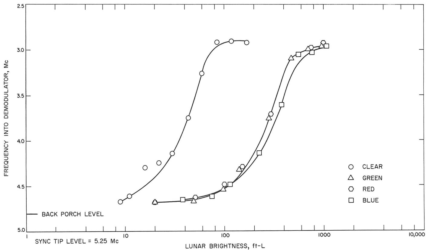
Fig. II-15. Surveyor III camera f/4 light-transfer characteristic for all filter-wheel positions: 600-line mode
