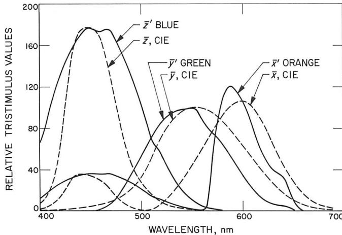
Fig. II-5. Camera-filter spectral response functions of Surveyor III camera, compared with CIE (Commission Internationale d'Eclairage 1931)
