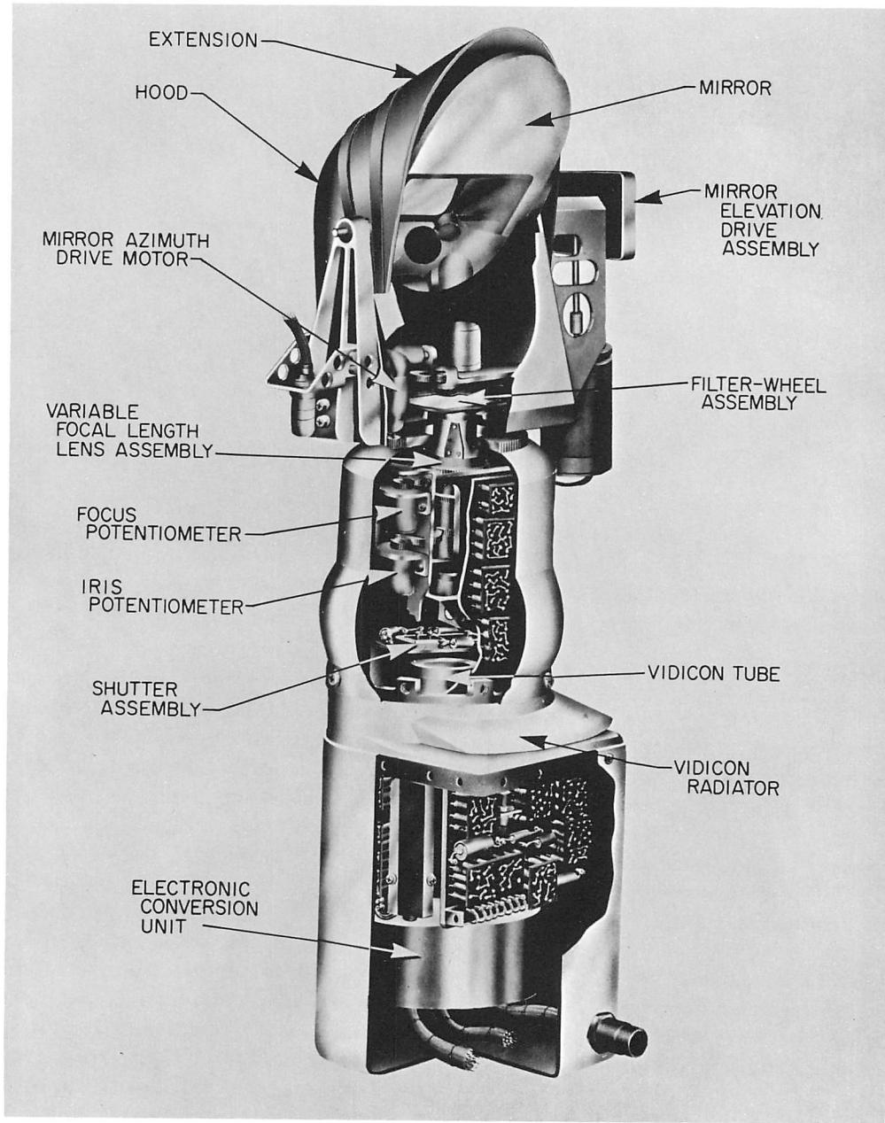
Fig. II-1. Cutaway view of survey camera
