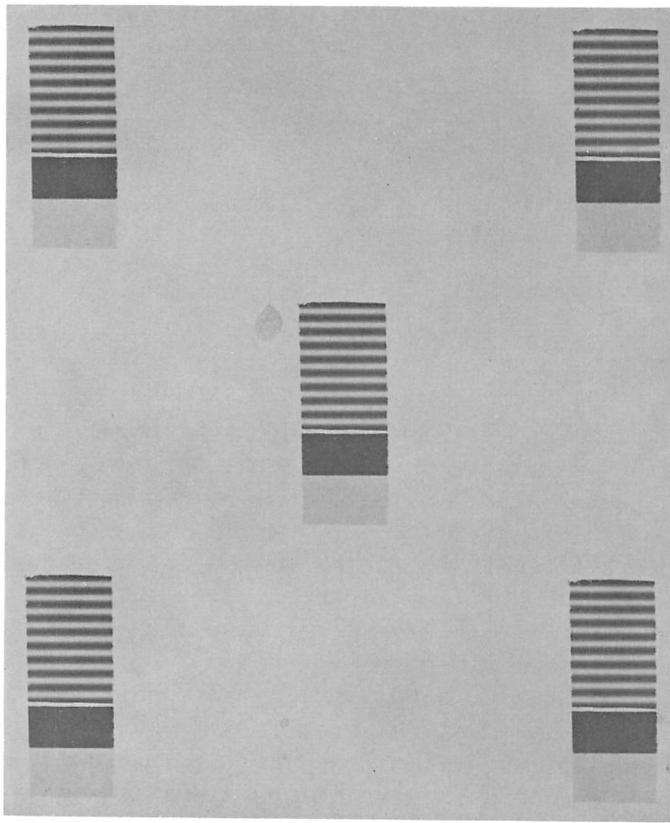
**Fig. II-11. Sine-wave target used to determine spatial frequency response of camera during calibration**
