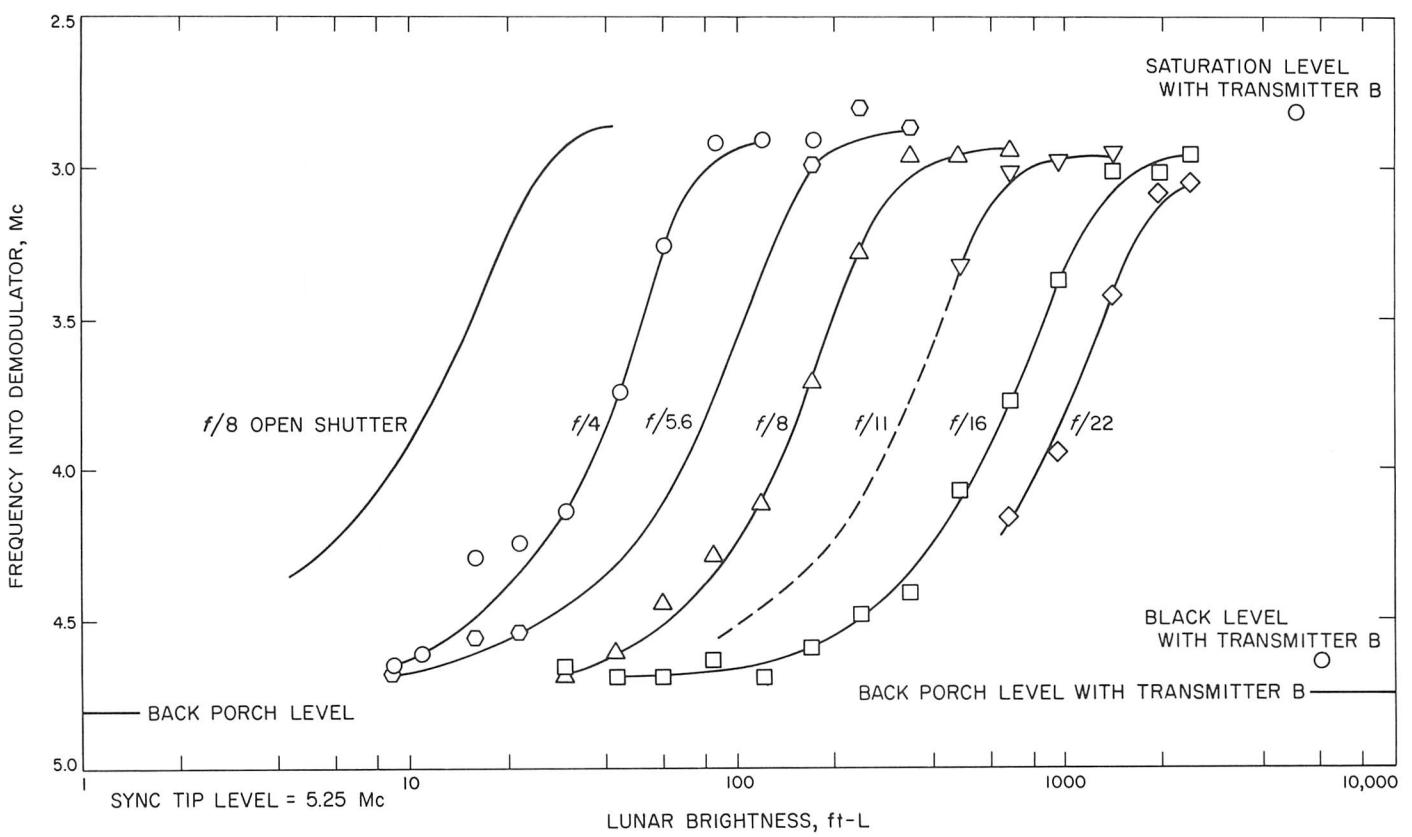
**Fig. II-13. Surveyor III camera light-transfer characteristic: 600-line mode**
