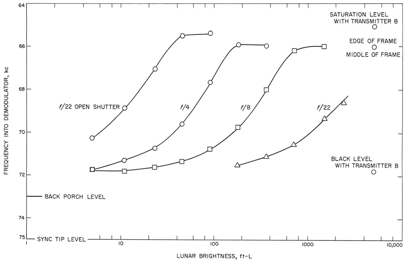
**Fig. II-14. Surveyor III camera light-transfer characteristic: 200-line mode**
