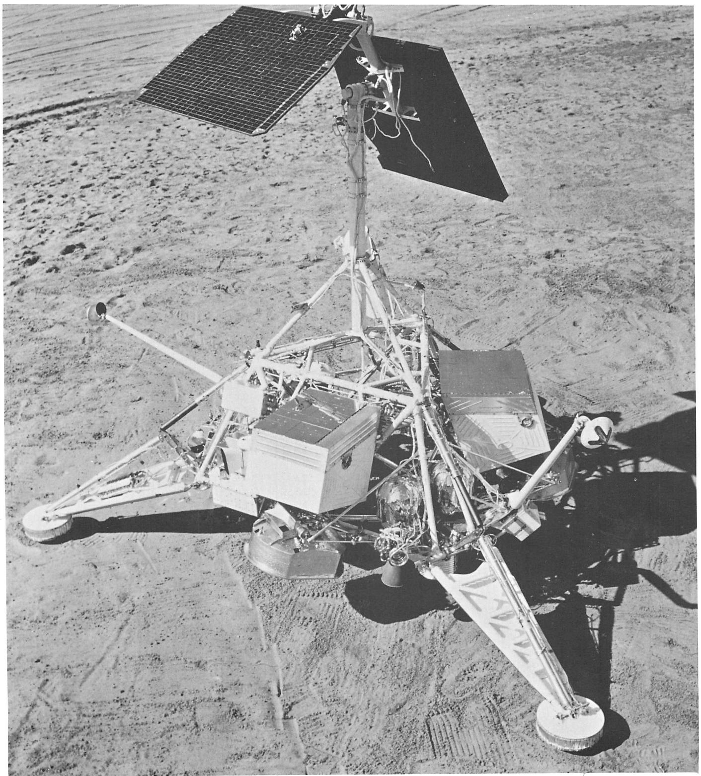
Fig. VI-2. Surveyor III spacecraft in landed configuration. Leg 1 is in foreground
