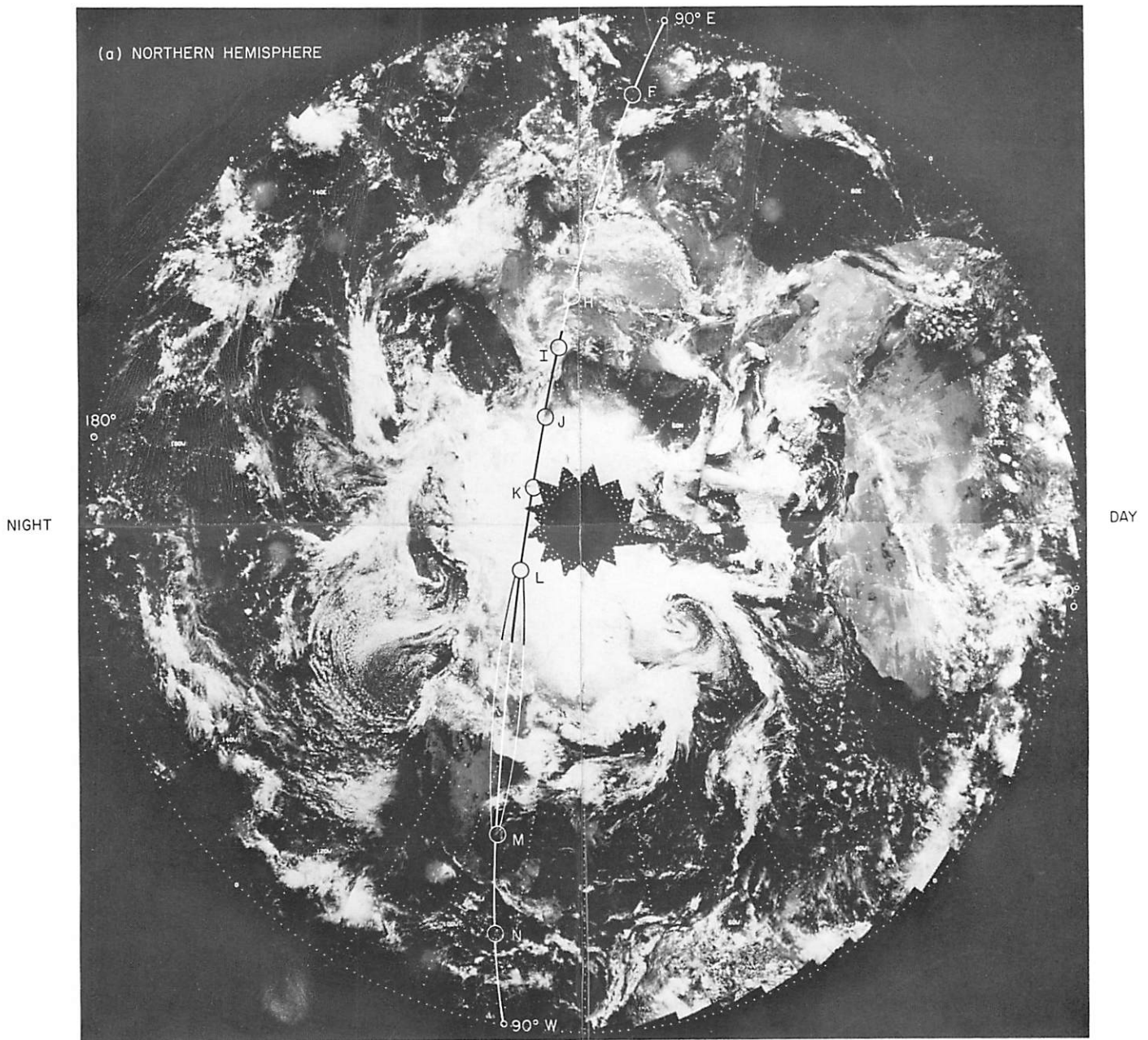
Fig. III-44. Stereographic mosaics of ESSA 3 pictures of (a) northern and (b) southern hemispheres of the earth. Pictures taken on the day preceding the eclipse. Bright areas are clouds and, in mountainous regions and the Arctic, snow fields; dark areas are clear. Note position of African continent, which may be seen in the clear areas on right-hand side of (a). Trace of limb of earth, as seen from the moon, and positions of beads and the bright region in the refraction halo of the earth observed in the second series of eclipse pictures taken by Surveyor III are shown by the white circles and lines that extend from 90° west to 90° east. Beads occur in areas that are largely clear. Letters beside symbols for beads correspond to letter identification of beads in Fig. III-43 (mosaic of ESSA 3 pictures provided through the courtesy of Dr. David S. Johnson, National Environmental Satellite Center, ESSA)
