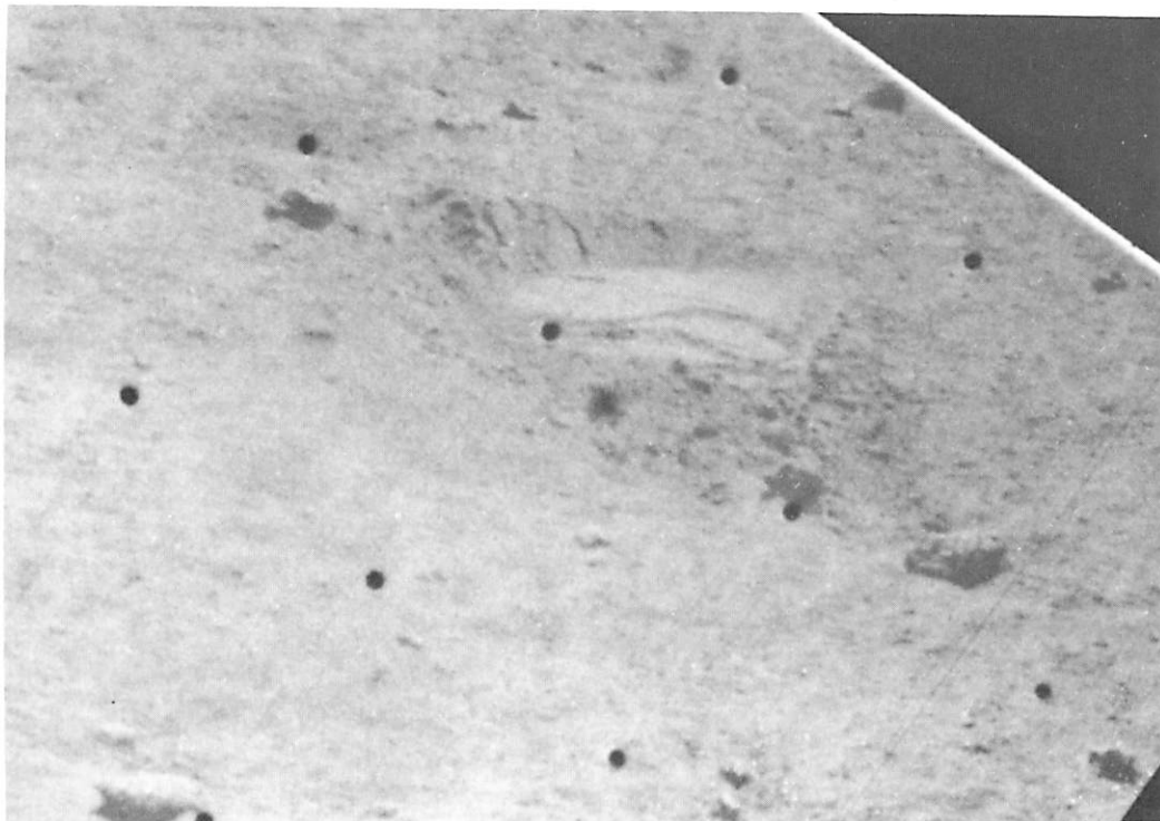
Fig. III-35. Narrow-angle Surveyor III picture, showing imprint in lunar surface produced by footpad 1 of the spacecraft during the second touchdown of the landing sequence. The imprint occurs on a small crater wall facing the camera, and the imprint is stepped down along several breaks toward the camera and toward the center of the small crater. The crater in which the imprint is formed is about 1 m across (Day 116, 08:37:36 GMT)
