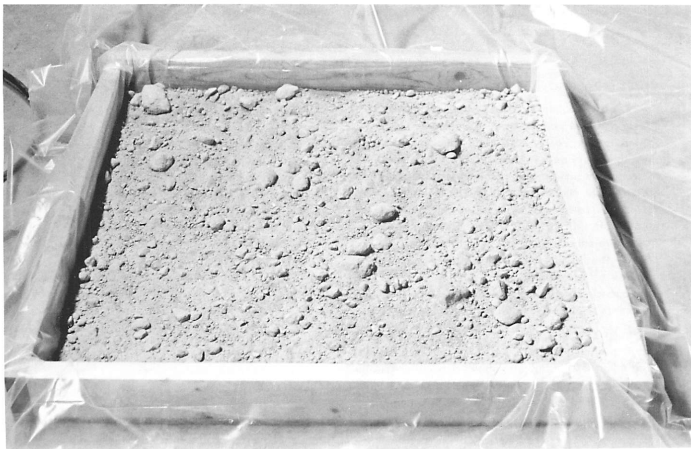
Fig. III-31. Sample of ash and pumice from volcanic ash flow deposited in the Valley of 10,000 Smokes, Alaska, during the eruption of 1912. Area of floor of box in which sample has been placed is 1 square meter. Coarsest fragments of pumice in sample are 4 to 5 cm across; finest grains identifiable in the picture are about 1 mm across
