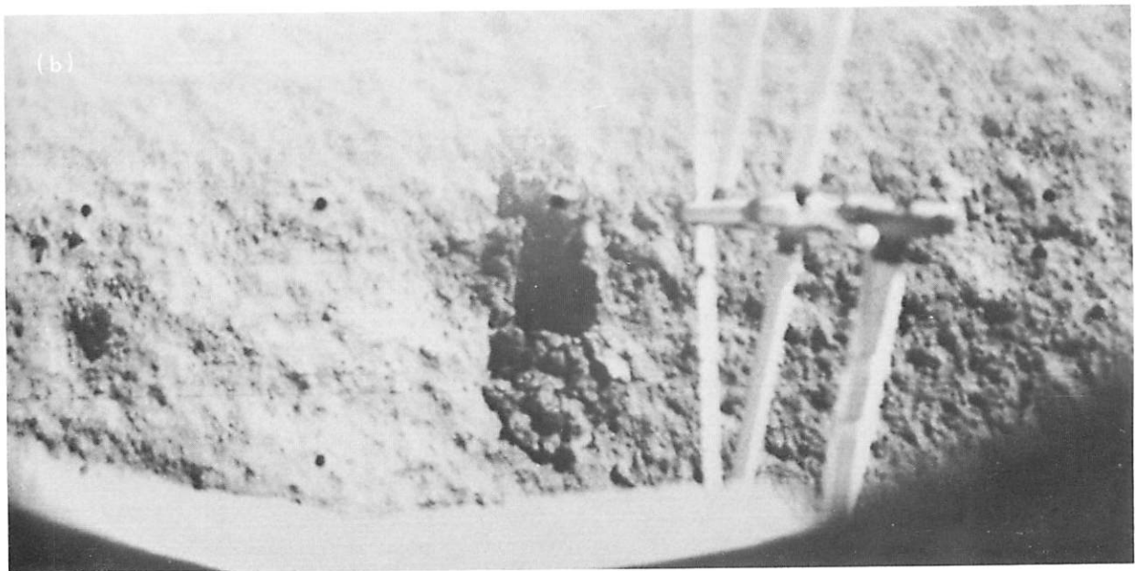
Fig. IV-24. Picture showing SMSS on Day 112: (a) before (05:07:01 GMT) and (b) after completion of first lunar surface bearing test (05:17:27 GMT)
