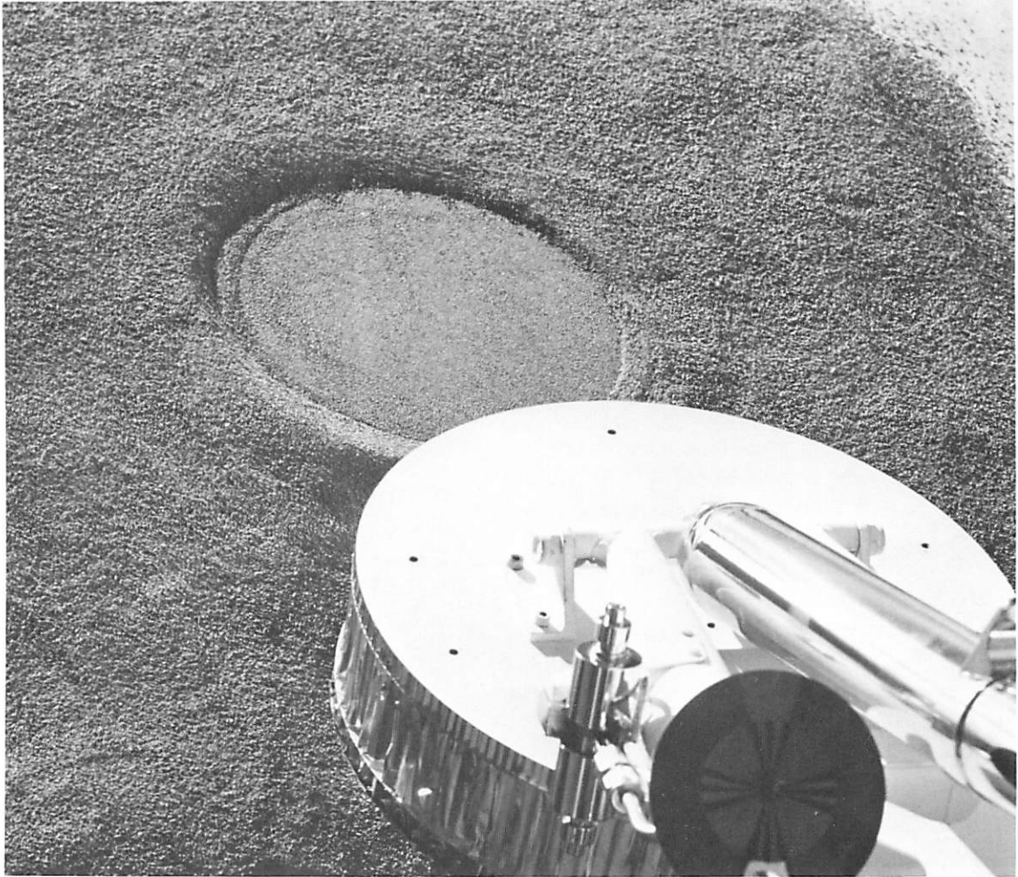
Fig. V-29. Laboratory simulation of footpad and imprint, made on earth with full-scale model of Surveyor . Surface material: crushed basalt, particle size in sand range only. Lighting angle similar to that of Fig. V-8
