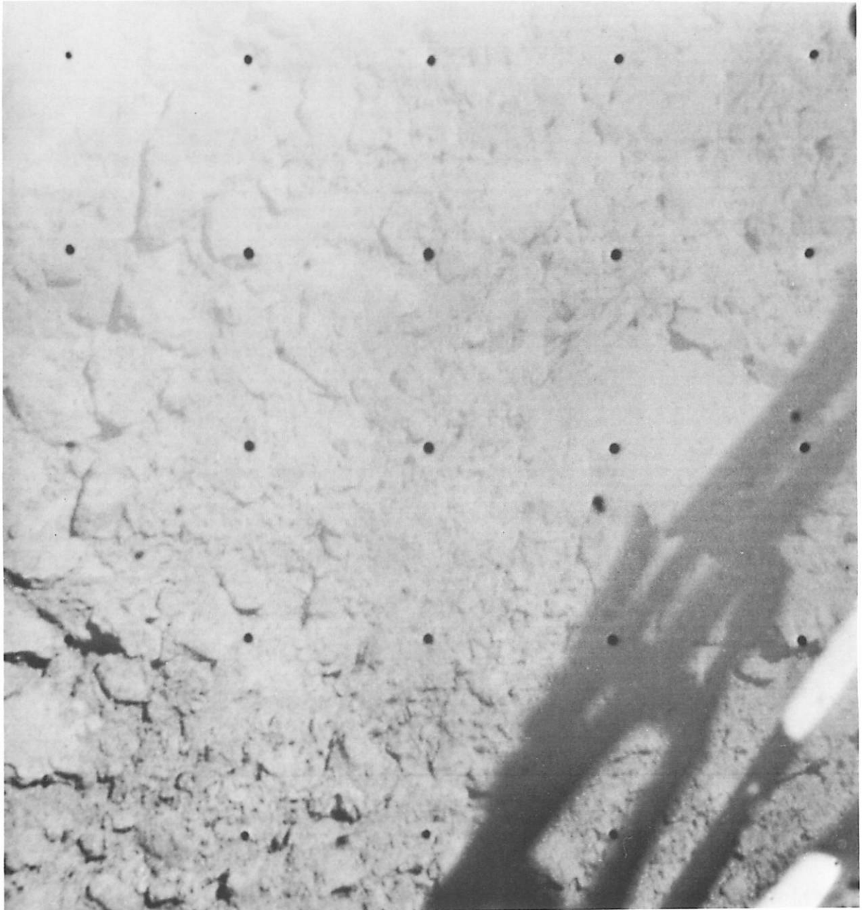
Fig. IV-30. Bearing test 4 impression in bottom of trench 3 at a depth of 5.1 to 7.6 cm below lunar surface. Depth of impression estimated from shadow. Broken-up soil from trenching operation is visible (Day 118, 13:35:22 GMT)
