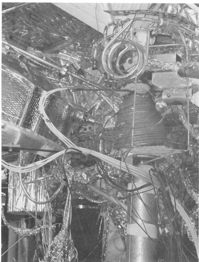
Fig. XV-13. Hot cone simulator
