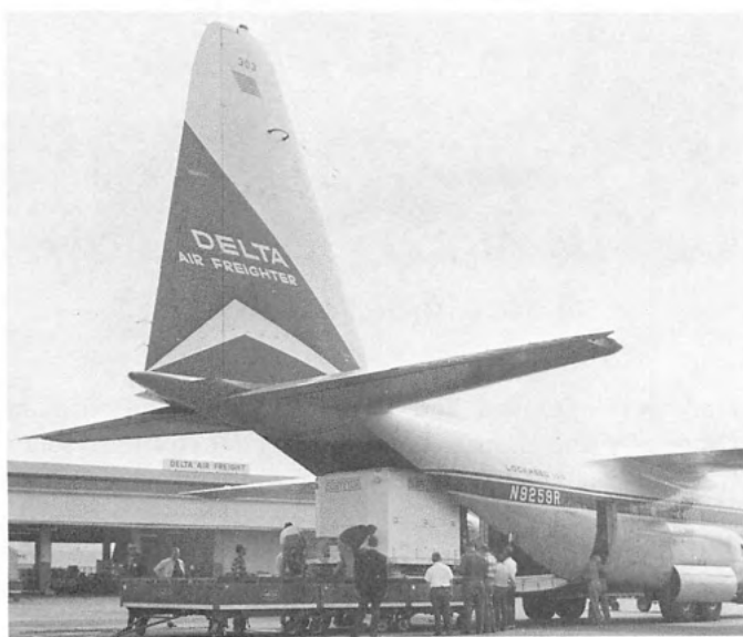
Fig. XI-19. Spacecraft loading for air shipment
