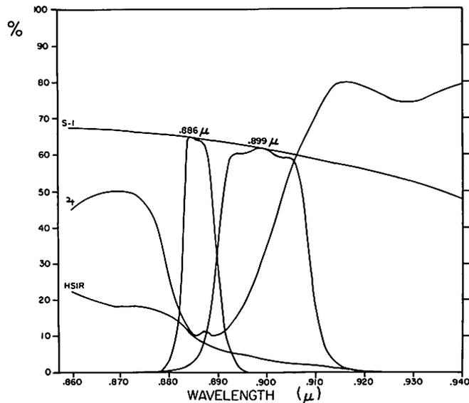
Fig. 3 Relative response of S-1 photo-emissive surface (RCA 6914), with 100% assumed at  $0.370\mu$ ; Sun/Jupiter intensity ratio for EZ, from Carl Pilcher (1971); relative sensitivity of Kodak HSIR film, with 100% assumed at  $0.400\mu$ ; and transmission of  $0.899\mu$  and  $0.886\mu$  filters
