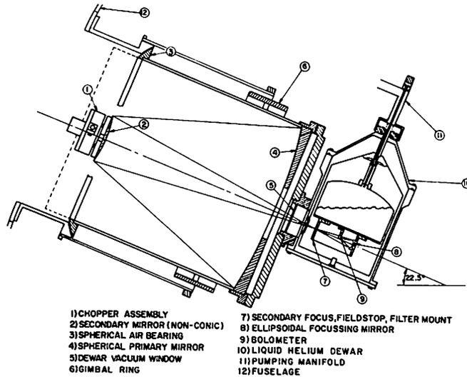
Fig. 47 Dr. Low's 12-inch open-port telescope equipped with liquid- $He$  cooled bolometer, for NASA Lear Jet, automatic guiding, 5 to 1000 $\mu$
