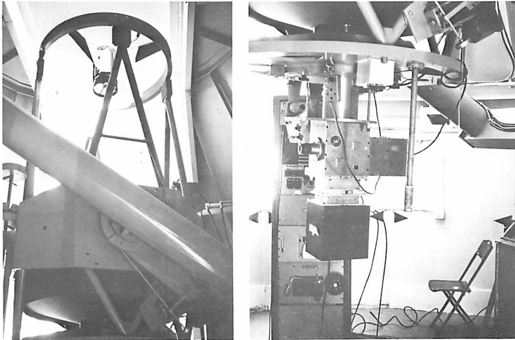
Fig. 17a&b 40-inch photometric telescope on Soldier Peak (el. 8570 ft, 2610 m) with photometer attached
