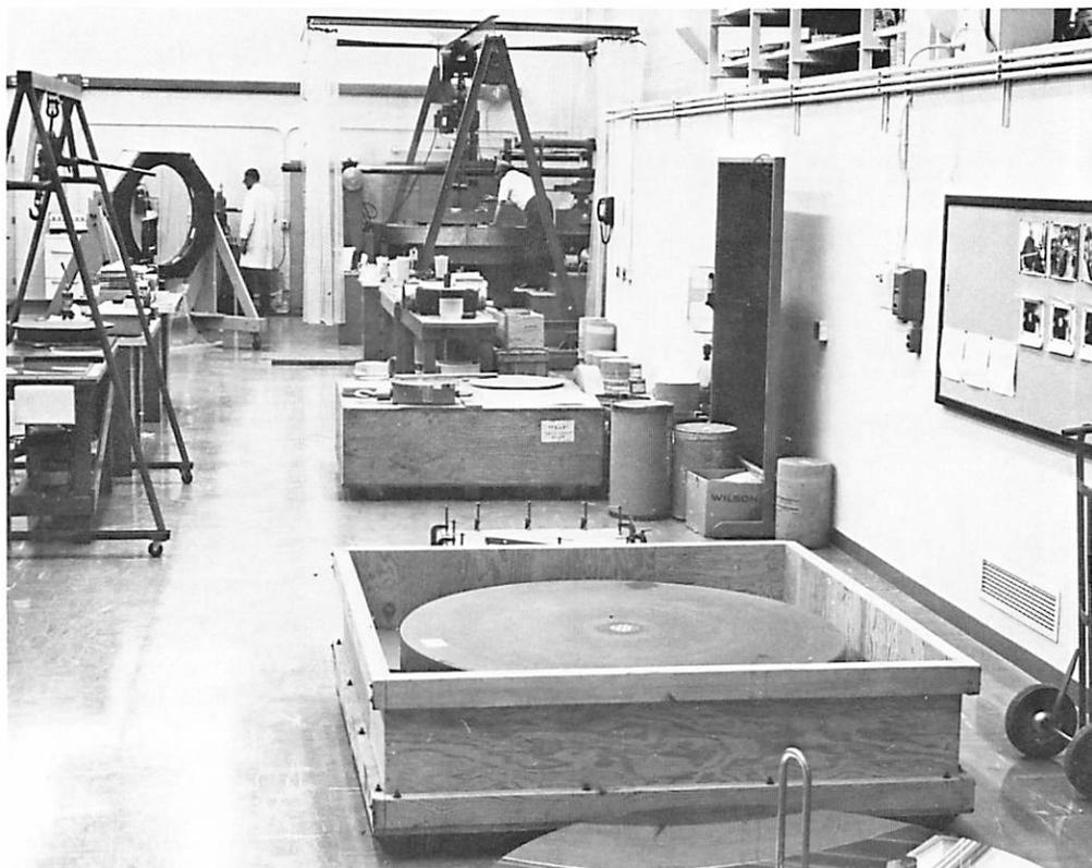
Fig. 3 Optical Shop, Lunar and Planetary Laboratory, Mr. R. L. Waland operating main tool; Mr. R. G. Crawford at second large tool. 60" metal mirror in foreground; U. of Minn. 60" blank in box. Forty-inch test flat and smaller grinding tools at left
