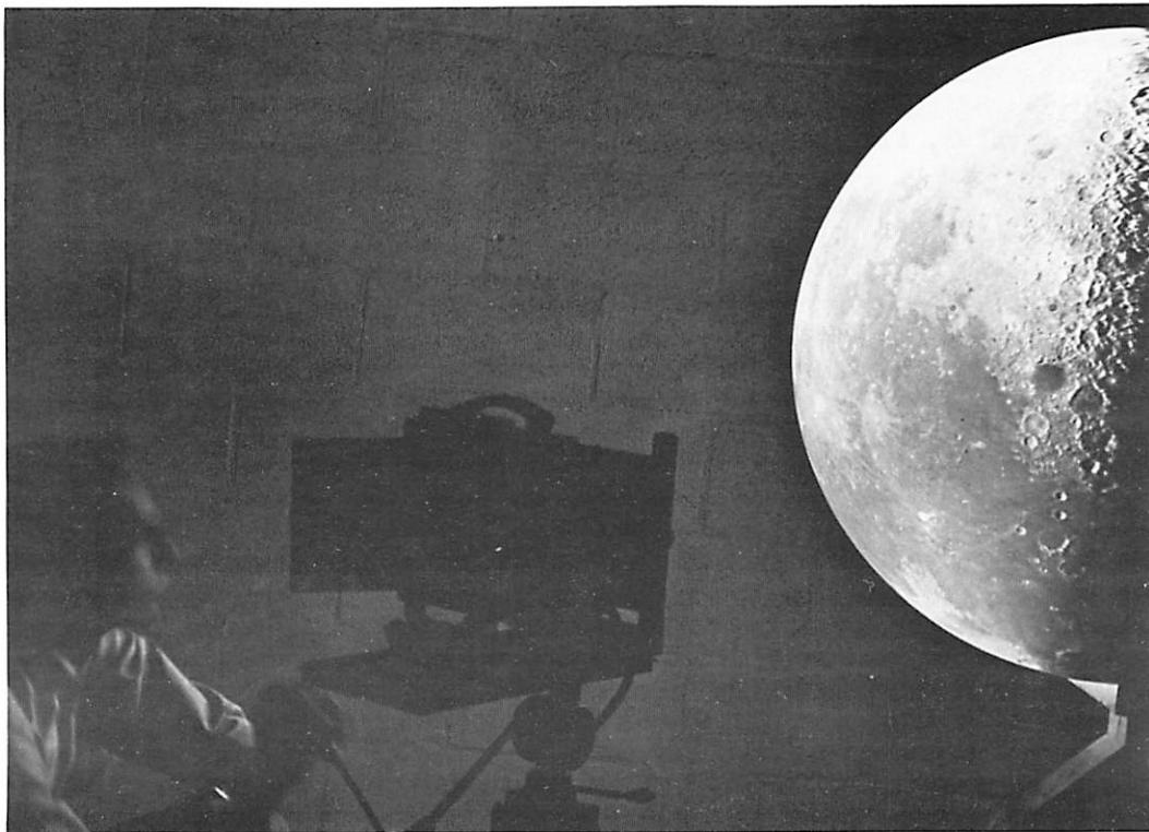
Fig. 8 Dr. W.K. Hartmann rephotographs lunar image projected orthogonally on hemisphere used in production of RECTIFIED LUNAR ATLAS
