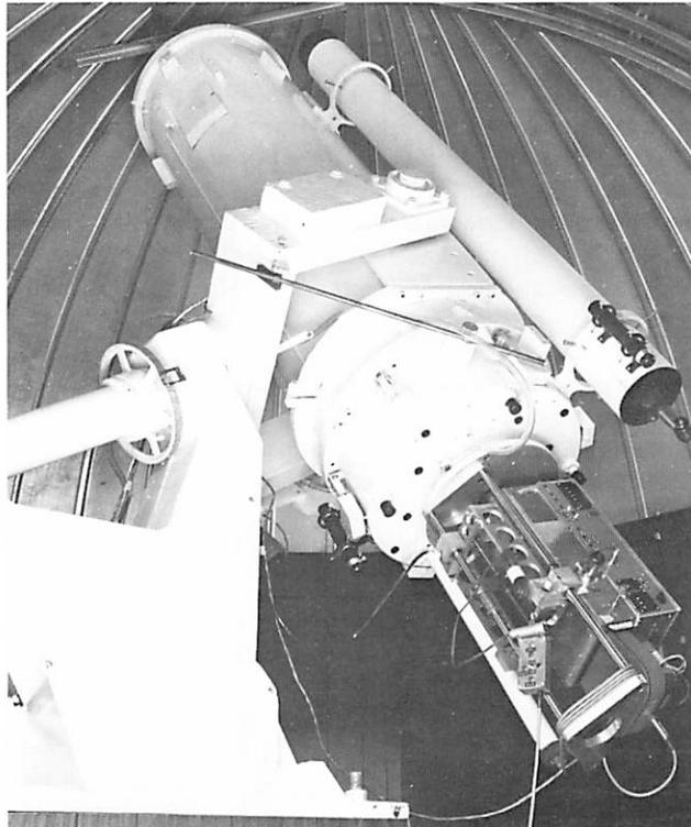
Fig. 39 21-inch planetary telescope on Tumamoc. The rod is clamped after a planetary series starts and has been most effective to quench vibrations in declination (wind, etc.)
