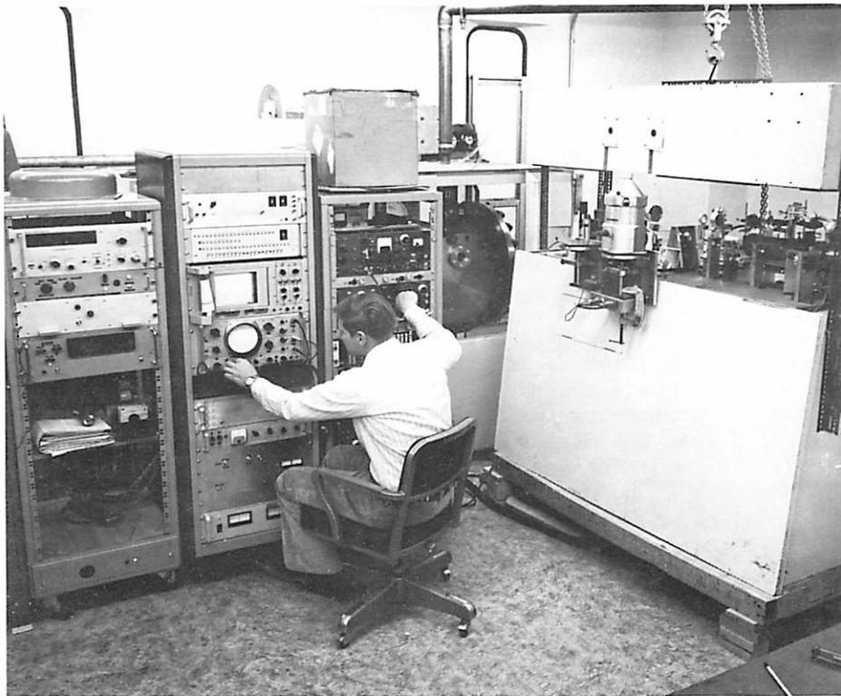
Fig. 4 Dr. H. Larson, operating modified Connes interferometer mounted at 130-ft Absorption Tube. Sunbeam as light source available behind Tube
