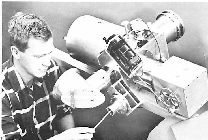
Fig. 46 Earlier model of Lear Jet IR spectrometer, hand-guided on Sun, by Dr. U. Fink
