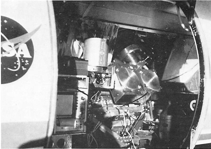
Fig. 45 Lear Jet with IR spectrometer using automatic guiding
