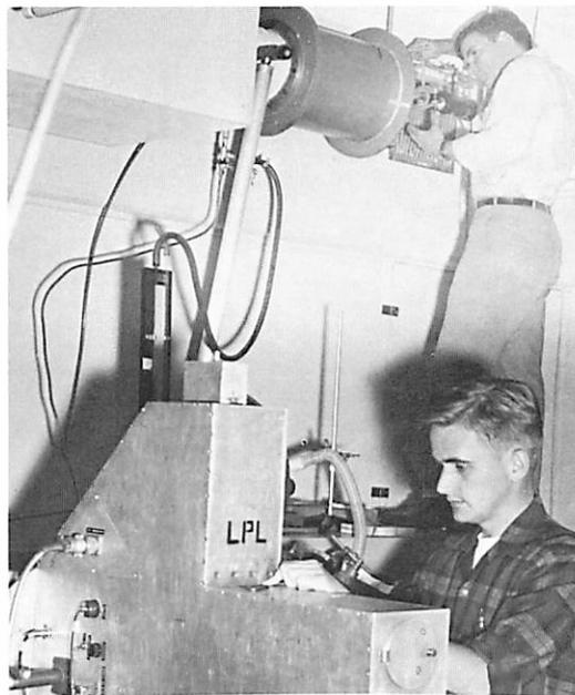
Fig. 5 T. Owen and D. Cruikshank adjusting Absorption Tube to simulate  $\text{CO}_2$  in Martian atmosphere using the "A" grating spectrometer (1964)
