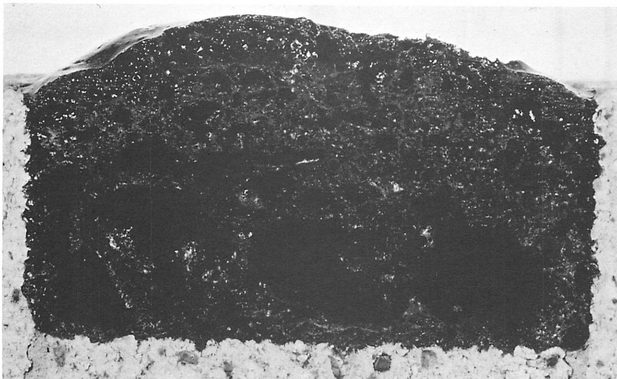
Fig. 2 Cross section of rock froth produced at p = 0.015 mm Hg. The low-density vesiculated structure is due to volatiles remaining in the melt at time of crystallization.
