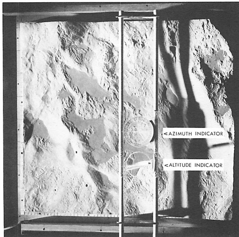
Fig. 4 Altitude and azimuth indicators, in place over model. Note model frame, also parallism of beams from Fresnel lenses. Shadows are very dark, as on moon.
