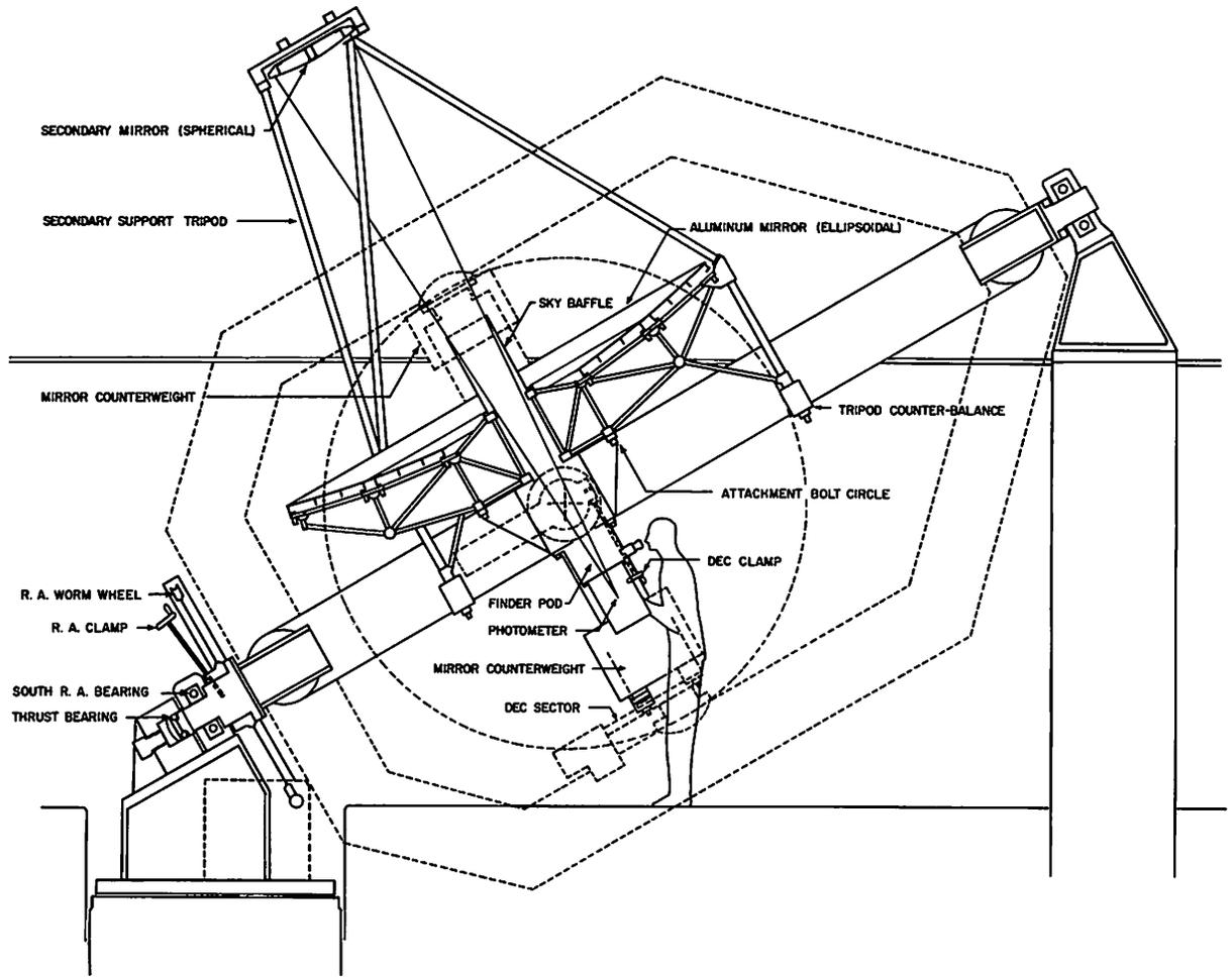
Fig. 2a. Preliminary design for a 10 ft. IR telescope, used at Cassegrain focus. Dotted line shows fork in 6-hour East position.
