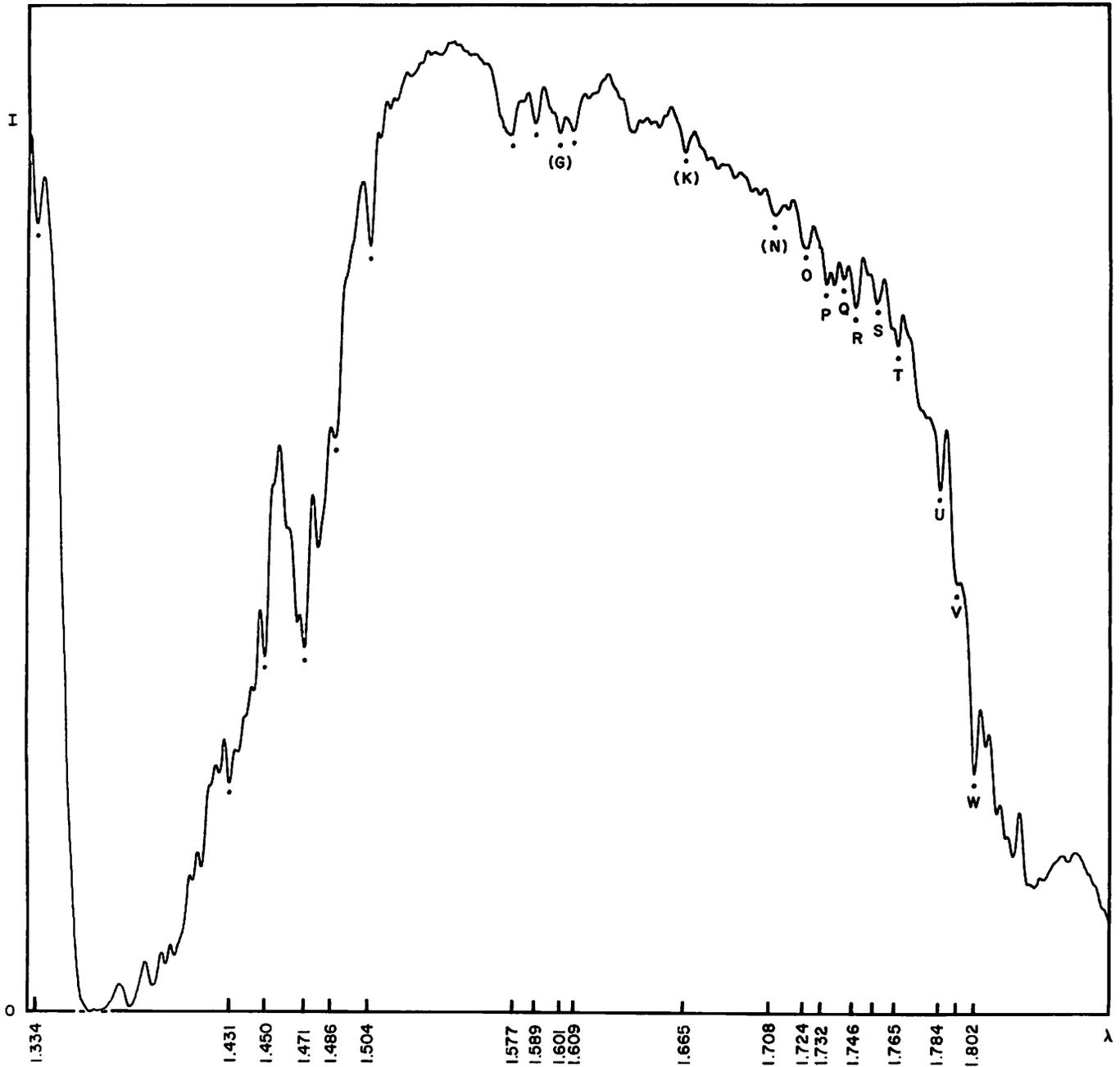
Fig. 8. Photographic reproduction of solar spectrum serving as comparison spectrum for  $\alpha$  Orionis, shown in Figure 7. Nearly all features shown are due to  $H_2O$ ; four dips near G are due to atmospheric  $CO_2$ .
