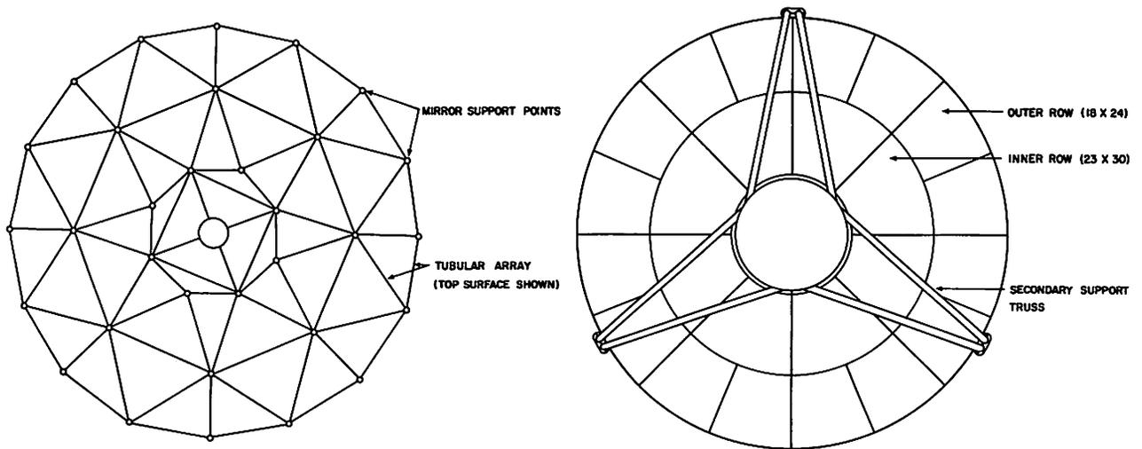
Fig. 2b. Left: Plan view of mirror support truss; each intersection provides collimation for one or more mirrors. Right: Plan view of mosaic mirror and secondary support system.
