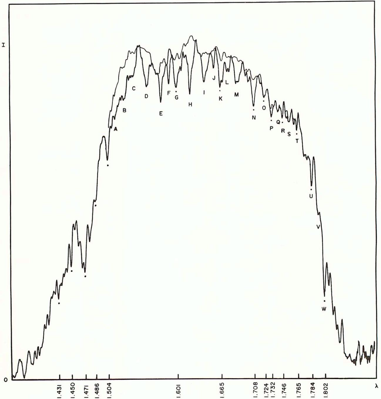
Fig. 7. Photographic reproduction of one of four almost identical spectra of  $\alpha$  Orionis, region 1.4-1.8 $\mu$ , obtained April 4, 1961, with 82-inch telescope. The wavelengths marked are those of telluric features, marked by dots, also shown in Figure 8. Upper fine curve corresponds to telluric spectrum recorded in Figure 8; difference between curves due to stellar absorptions, which appear prominent from A to S. Compare Figure 10.
