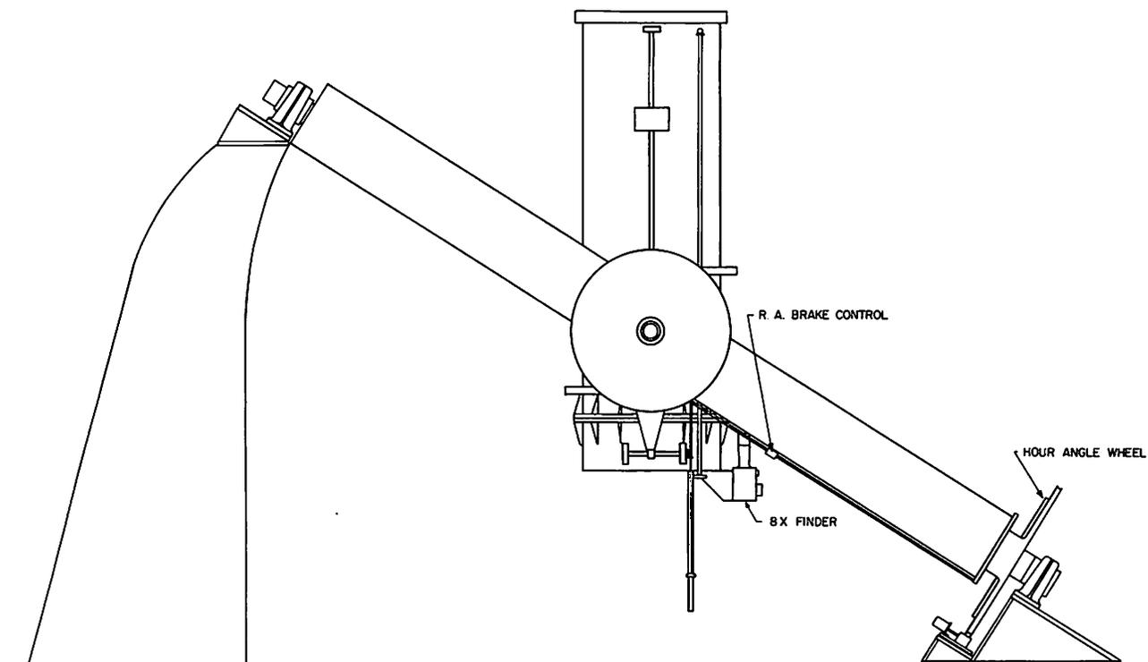
Fig. 3a. Design drawing of 21-inch telescope by W. L. Richards Co. of Austin, Texas, manufacturers of this instrument.
