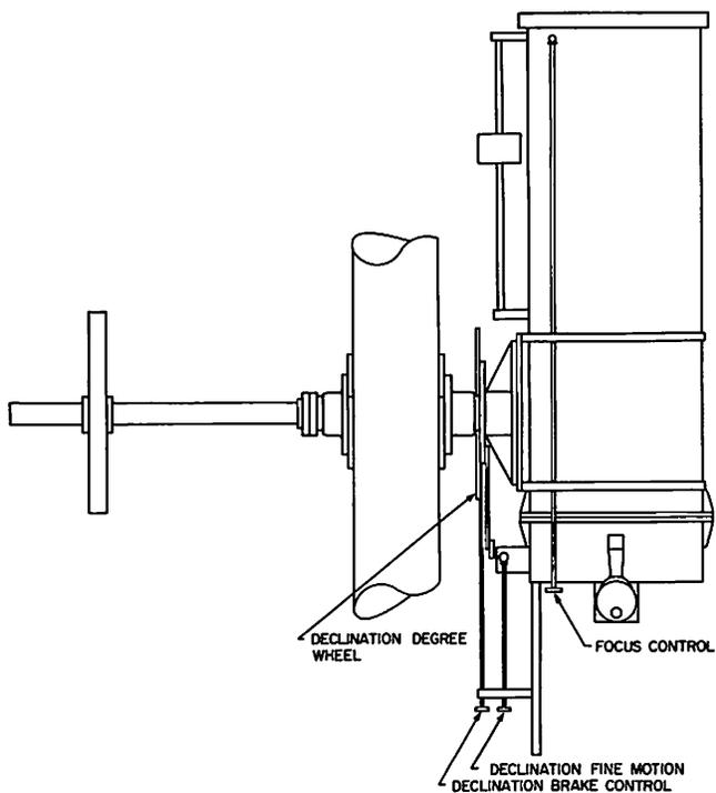
Fig. 3b. Design drawing of 21-inch telescope by W. L. Richards Co. of Austin, Texas, manufacturers of this instrument.
