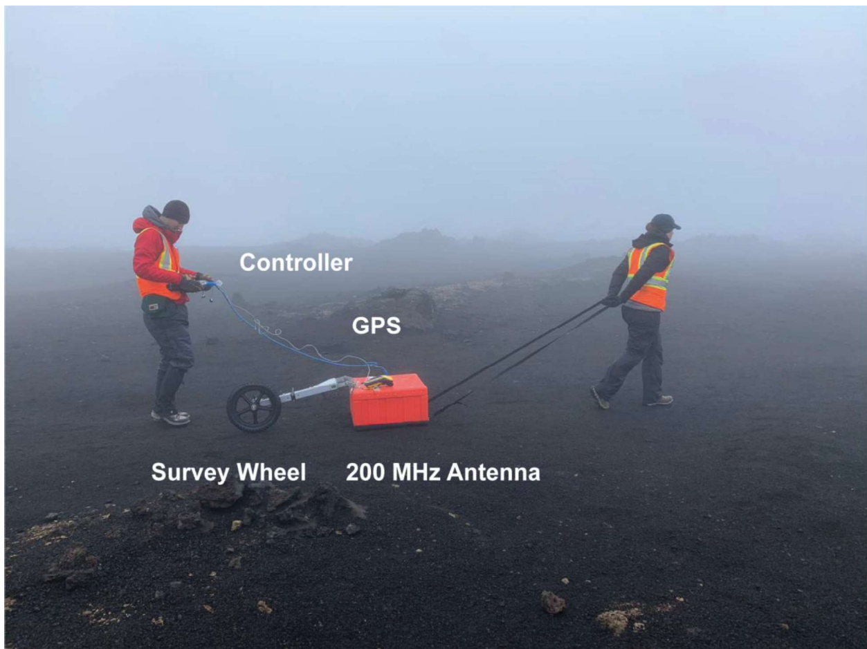
Figure 3. Example of the GSSI GPR setup. The 200 MHz antenna (orange box) is pulled by a strap connected to the box itself with a calibrated survey wheel attached to measure distances. The Trimble Geo7x GPS is attached to the survey wheel mount. One person pulls the antenna forward while the other walks behind holding the controller and monitoring the output in real-time.
