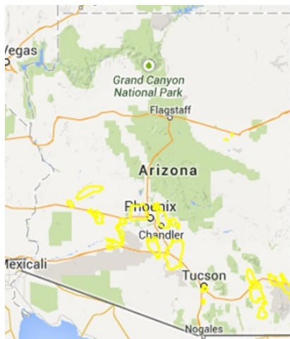
Figure 9. Map of Arizona areas of active land subsidence based on InSAR data. Credit: Arizona Department of Water Resources.
