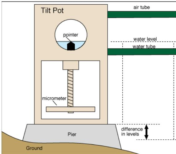
Fig 5. The schematics of such a tiltmeter.
