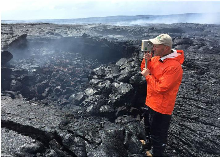
Fig 9. HVO geologist conducts a VLF (very-low-frequency) electromagnetic survey across an active lava tube to determine the cross-sectional area of the lava stream coursing through the tube, Kilauea, Hawai'i.
