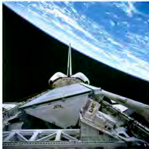
Spaceborne Imaging Radar-C/X-band Synthetic Aperture Radar (SIR-C/X-SAR) in the payload bay of space shuttle Endeavour. Because it uses SAR, it can quite easily be placed in orbit. 1994. Image credit: NASA/JPL
