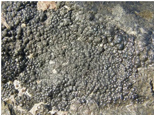
Uraninite, also known as pitchblende, is the Uranium ore found in breccia pipes.
