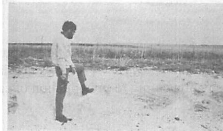
Figure 3-1. Soft powdery caliche in situ , Western Transvaal, Southwest Africa (courtesy F. Netterberg).
