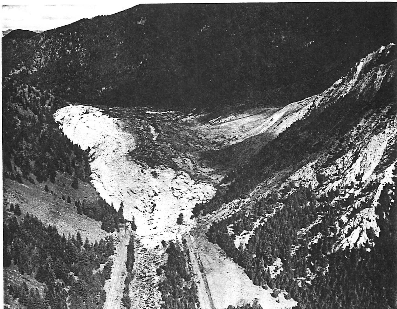
FIGURE 54.—Madison Slide, upstream view showing the west edge of the slide debris, blocked highway, and dry river bed below the slide. U.S. Forest Service photograph.
