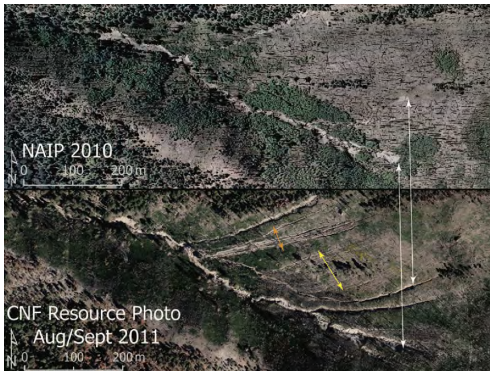
Fig. 3: Example of post fire erosion after the Horseshoe 2 fire including rills (orange), new gullies (yellow), and older gullies from the 1994 fire (white) (Youberg et al. 2013).
