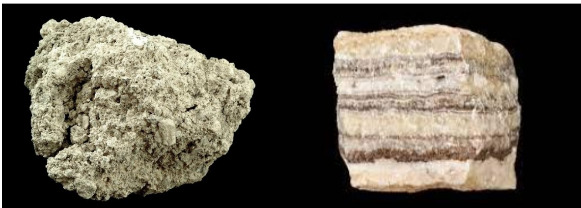
Figure 2: Tufa (left), which forms in cold-to-warm aqueous conditions. Travertine (right), which forms in warm-to-hot aqueous conditions.
